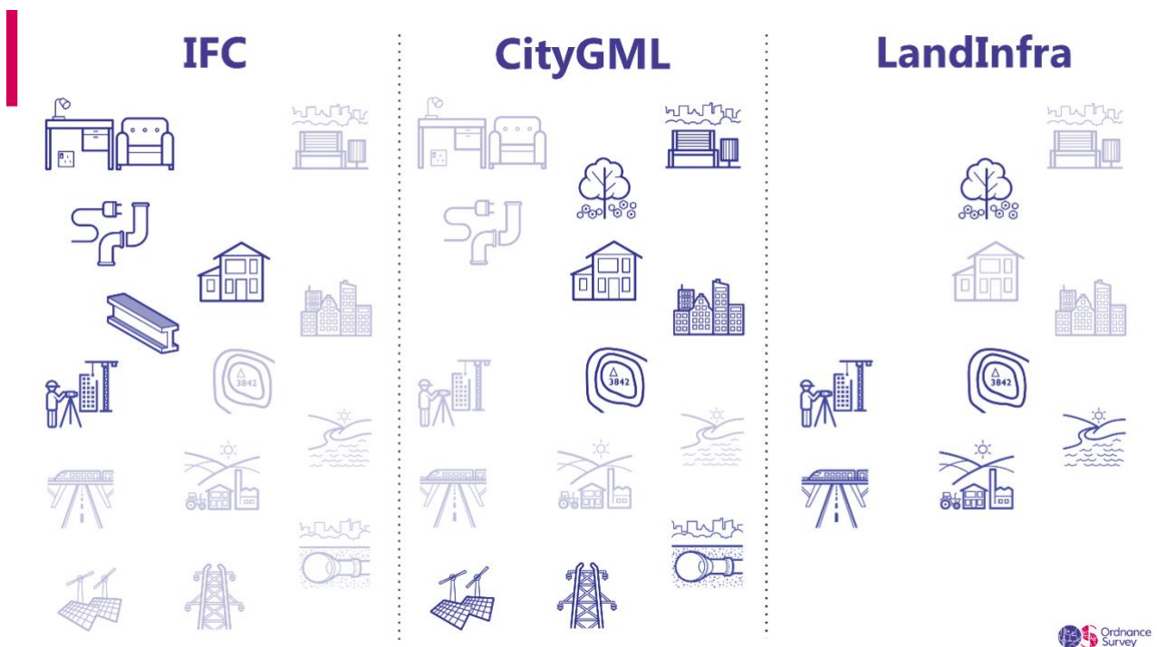
Figure 1 - Thematic coverage of the three data standards. Dark shading indicates strong coverage, light shading weaker coverage (or under development) and no shading implies no known coverage. The object icons are ordered approximately; the intention is to cluster by theme and represent finer spatial scales nearer the top.
