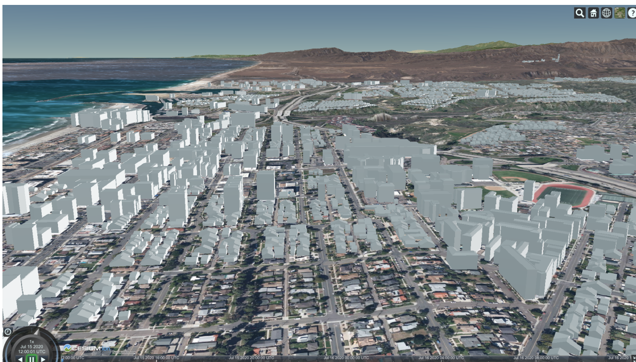
Figure 10. CesiumJS client accessing Camp Pendleton data from GNOSIS Map Server as 3D Tiles generated on-the-fly
