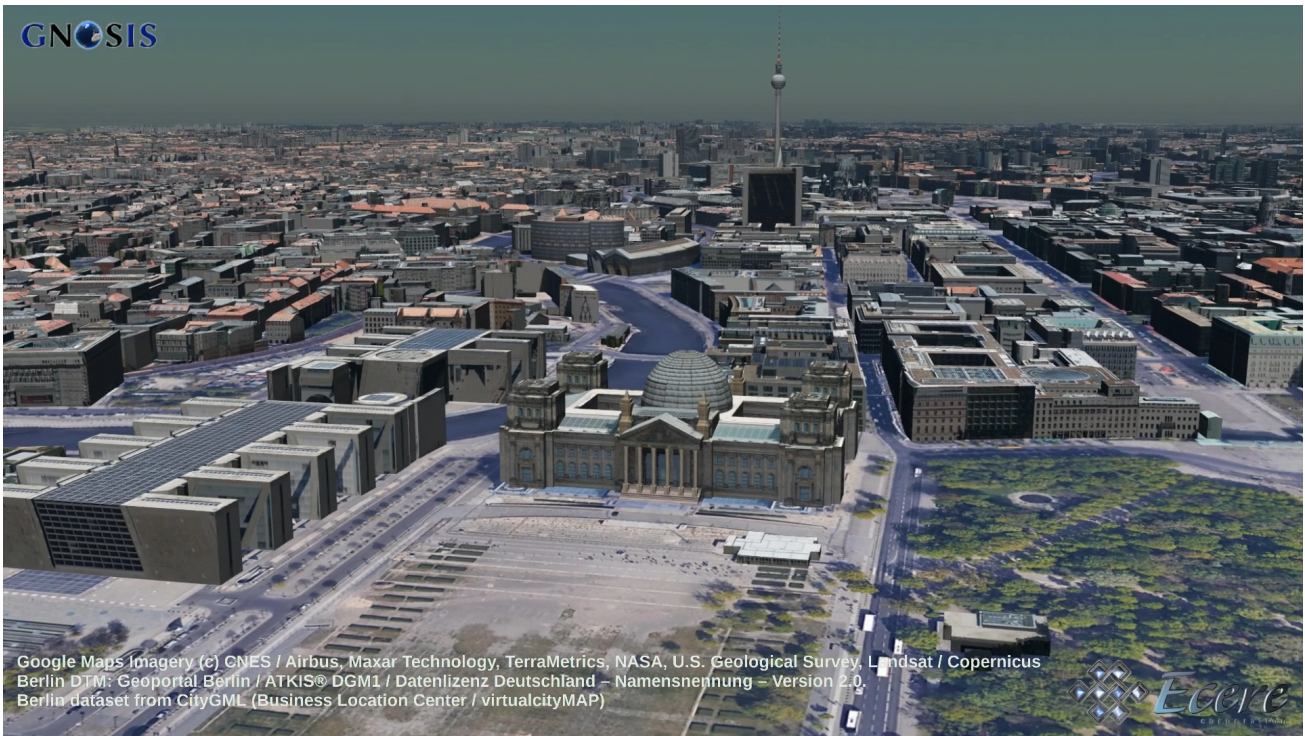
Figure 42. Textured dataset of Berlin originating from CityGML being served as 3D Tiles by virtualcityMAP from virtualcitySYSTEMS (additional non-participating service tests)
