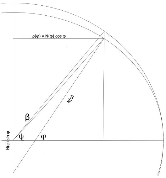
Figure 1 – Reduced latitude " $\beta$ ", geocentric latitude " $\psi$ ", and geodetic latitude " $\phi$ ". (larger eccentricity for emphasis)
