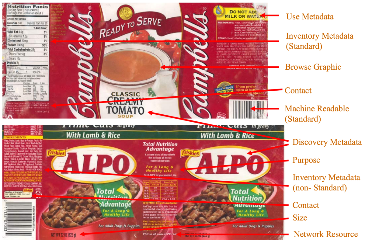
Figure 2: More advanced set of metadata items on products - human and machine readable, standard and non-standard representations
