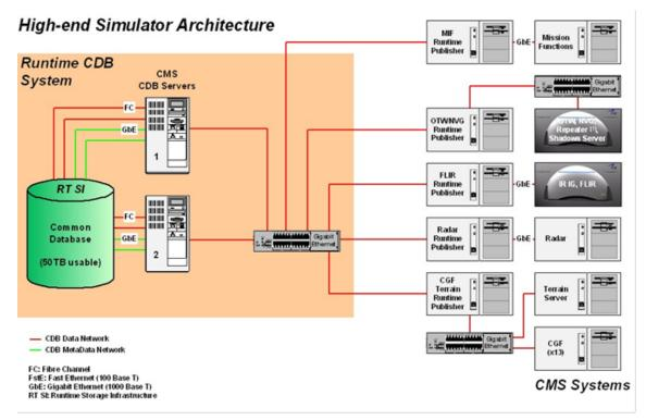
Figure 3: Typical Implementation of CDB Standard on High-end Simulator
