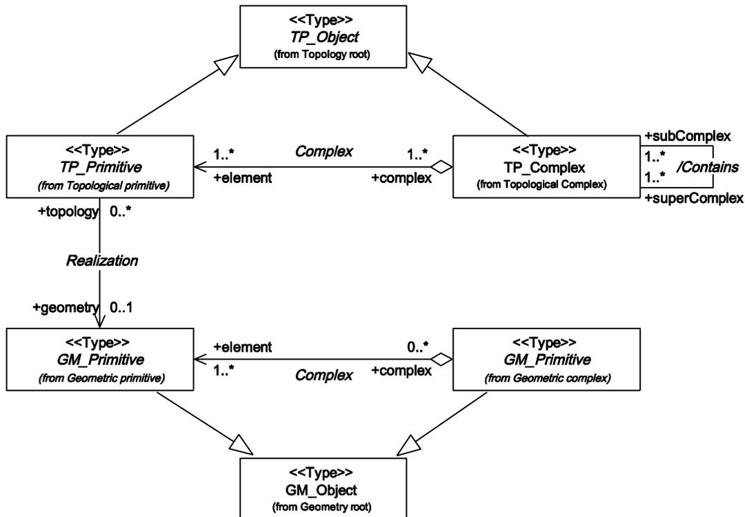
Figure 32 — Relationship between geometry and topology
