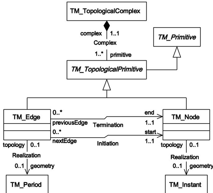
**Figure 42 — Profile of temporal topology adapted from ISO 19108**
