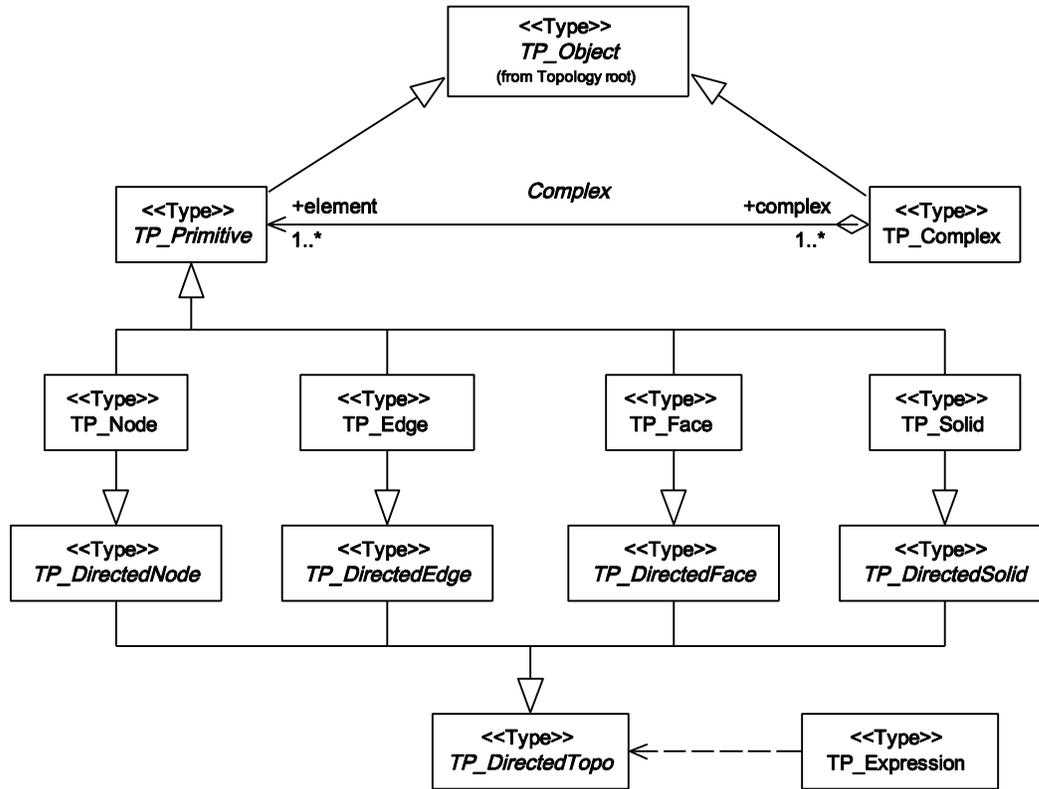
Figure 31 — Topologic primitives
