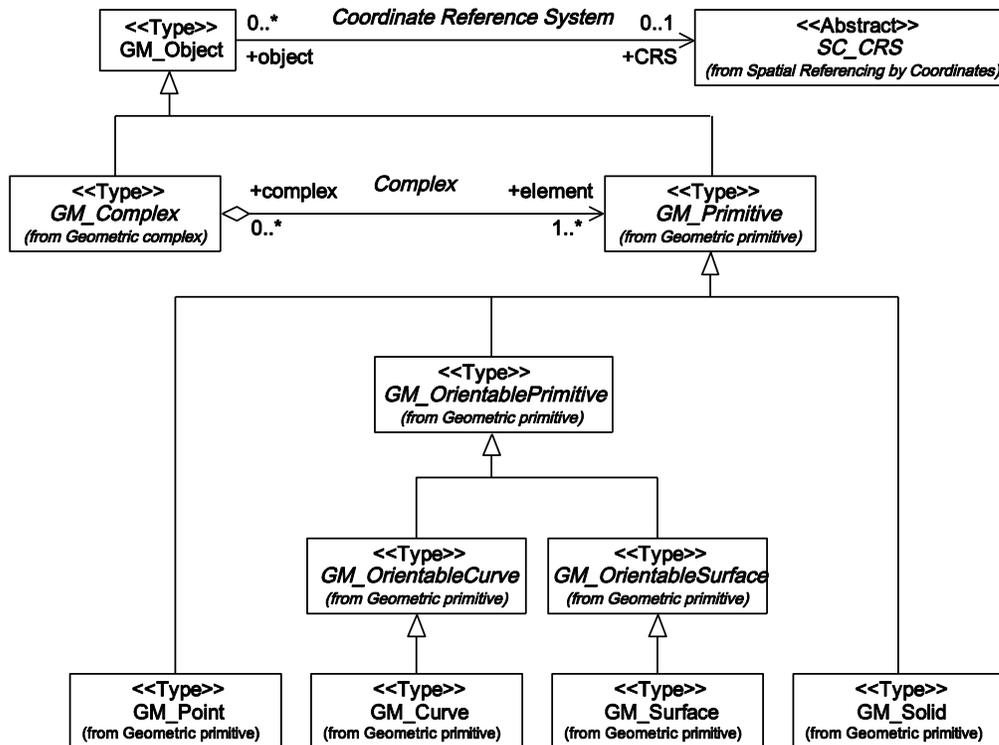
Figure 10 — Geometric primitives
