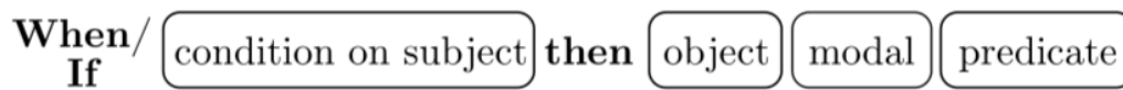
Figure 22: Proposed structure of a conditional sentence consisting of 4 structural elements for formulating conformance requirements. (adapted from van Walstijn (2015))
