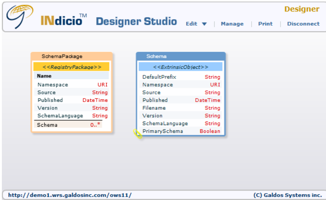
Figure 4 -- Model extensions for schema management
