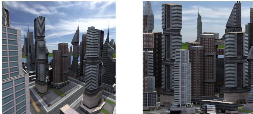
Figure 13: Examples of perspective (left) and orthographic (right) projections.
