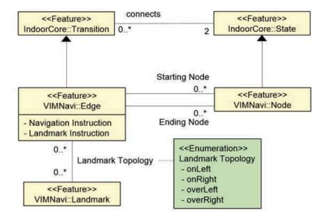
Figure 5 — Extension of IndoorGML Core Module for VIM
