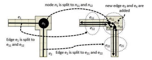
Figure 6 — Splitting Nodes and Edges
