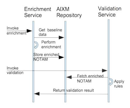
Figure 11 – Integrated Enrichment and Validation Service
