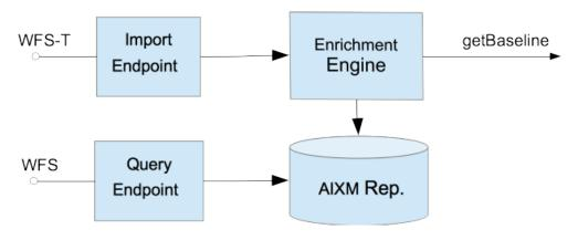
Figure 8 - Enrichment Service Component Diagram
