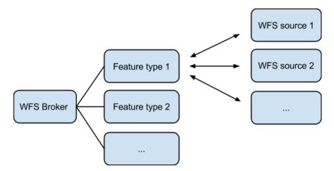
Figure 13 - High-level architecture of the WFS-based Data Broker
