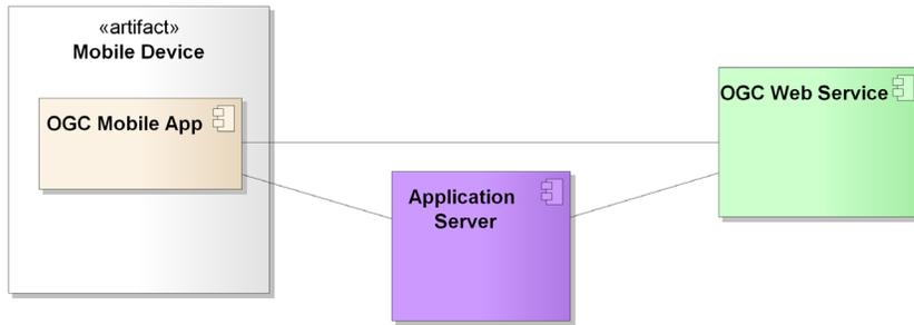
**Figure 2: OGC Enabled Mobile App to OGC Web service communication**
