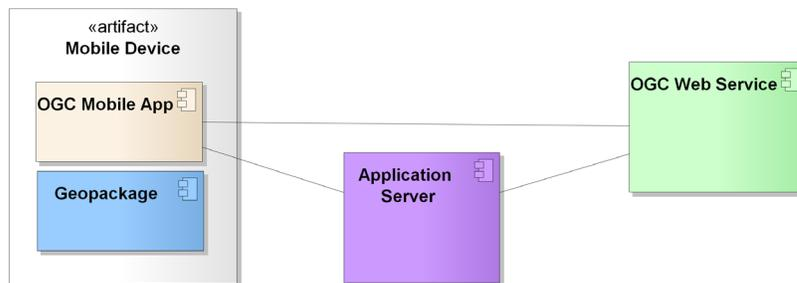
**Figure 4: OGC Enabled Mobile App combined data handling**
