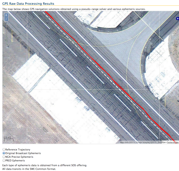
Figure 10. Close-up results for Use Case 1: Original Broadcast Ephemeris. (track show in red)
