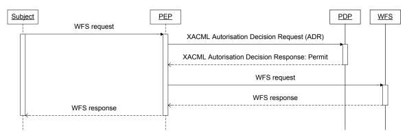
Figure 12: Information flow in case of a permit XACML authorization decision response without rewrite-obligations
