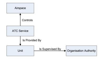
Figure 22: Relationship of relevant AIXM features used in determining Controlling Agency and Using Agency for an airspace.
