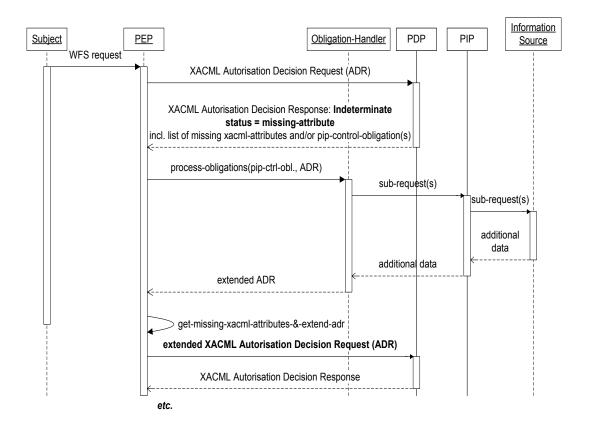
Figure 16: Information flow in case of an indeterminate response with missing-attribute information and/or PIP-control-obligations
