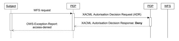
Figure 13: Information flow in case of a deny XACML authorization decision response without rewrite-obligations
