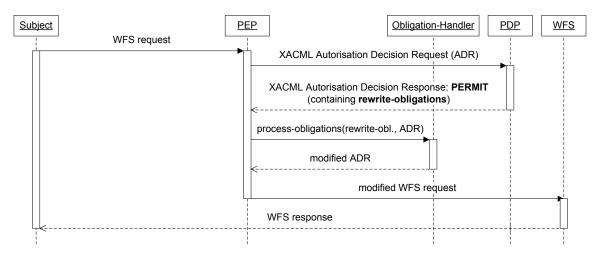
Figure 14: Information flow in case of a permit XACML authorization decision response with rewrite-obligations
