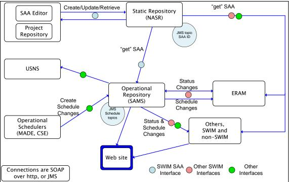
Figure 5-1. Diagram of SWIM SAA systems and interfaces.
