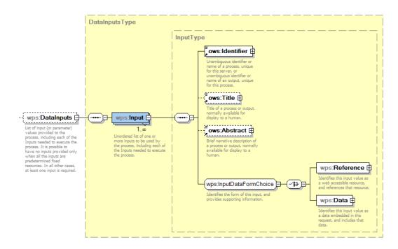
Figure 4 — Standard WPS Input Schema Diagram
