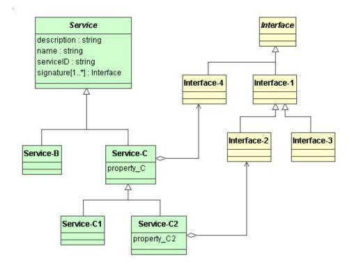
Figure 17 - Service and Interface Types
