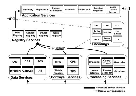
Figure 18 - The OWS Service Framework (OSF)
