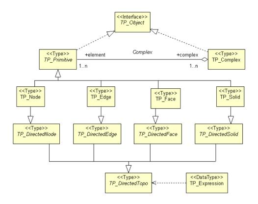
Figure 8 - Topological Class Diagram
