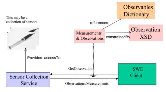
Figure 27 - Sensor Collection Service concept
