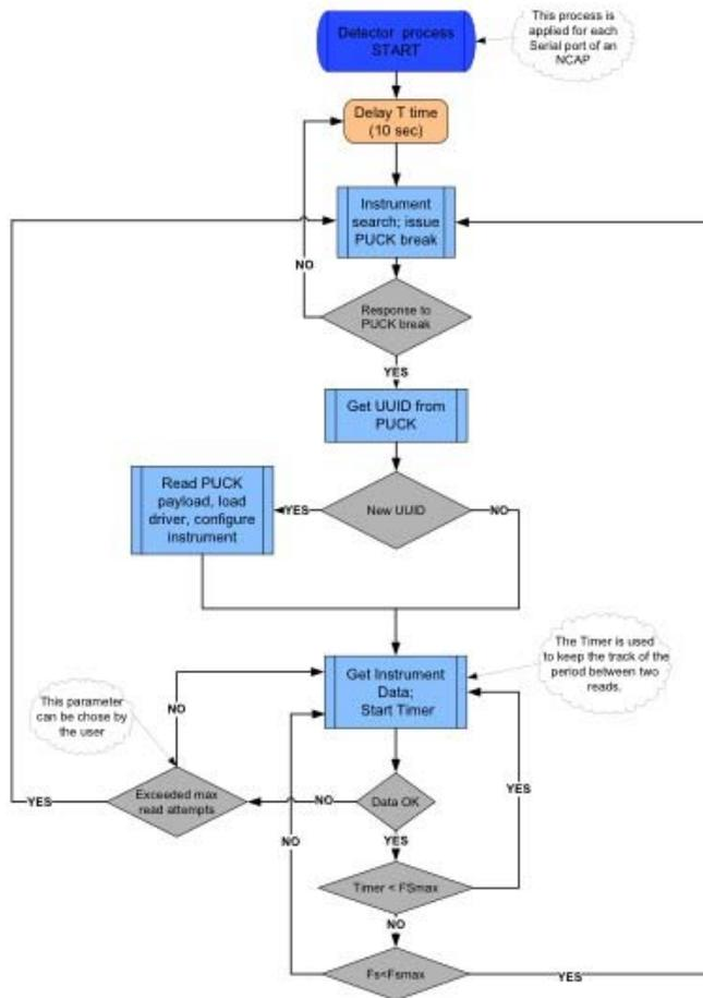
Figure PUCK-5: Automated instrument detection algorithm developed at UPC-SARTI .
