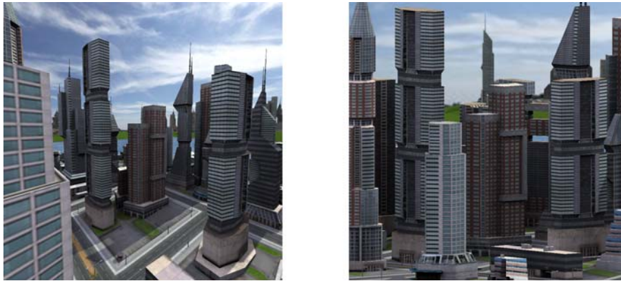
Figure 9 — Examples of perspective (left) and orthographic projections (right).
