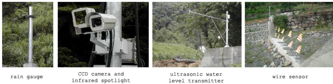
Figure 6 Different sensors deployed at a fixed monitoring stations
