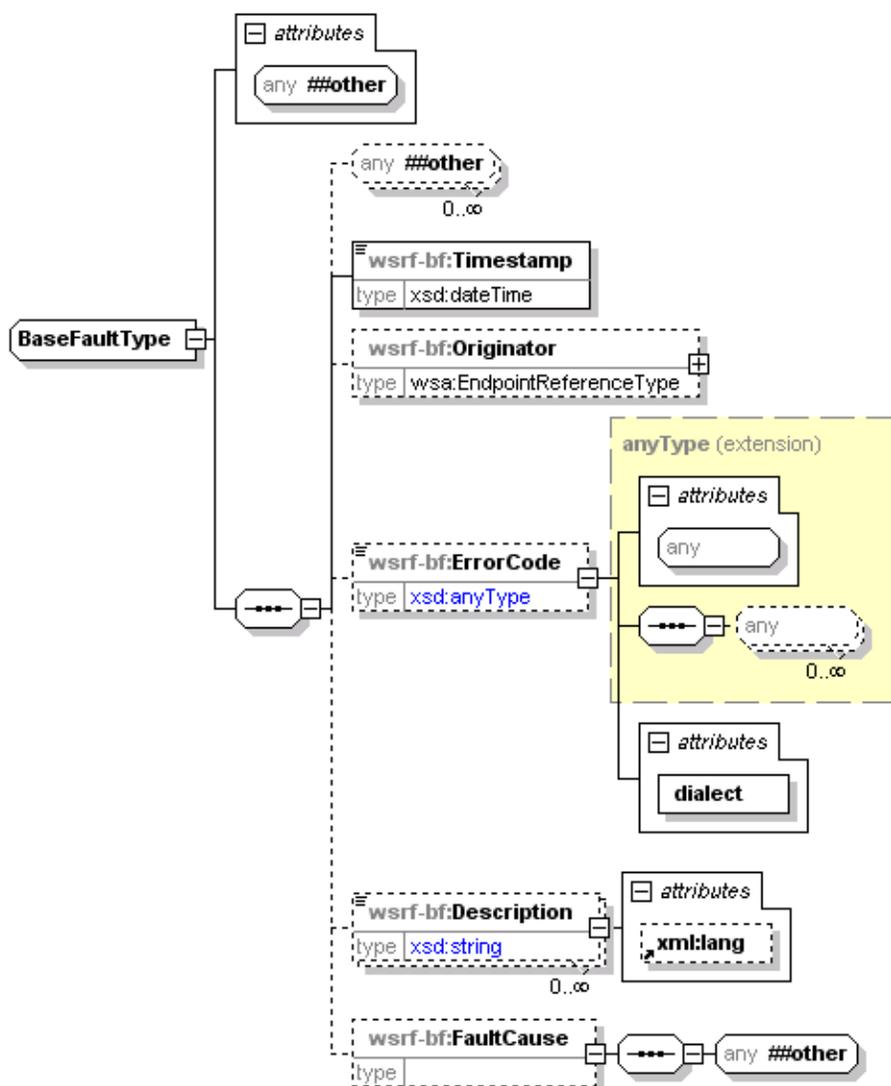
Figure 57 - WS-BaseFaults BaseFaultType in XMLSpy notation
