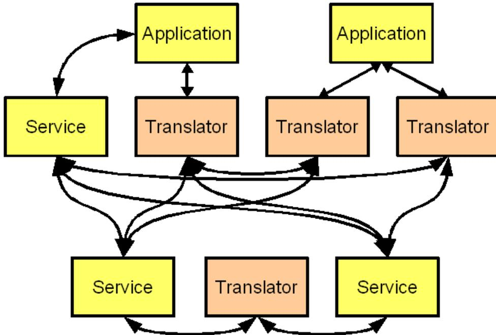
Figure 46 - Distributed system without an ESB
