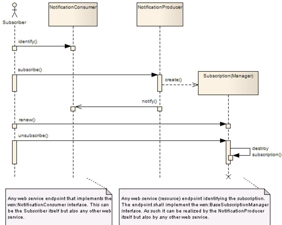
**Figure 66 - Basic Interactions in Pub/Sub using WS-Notification**
