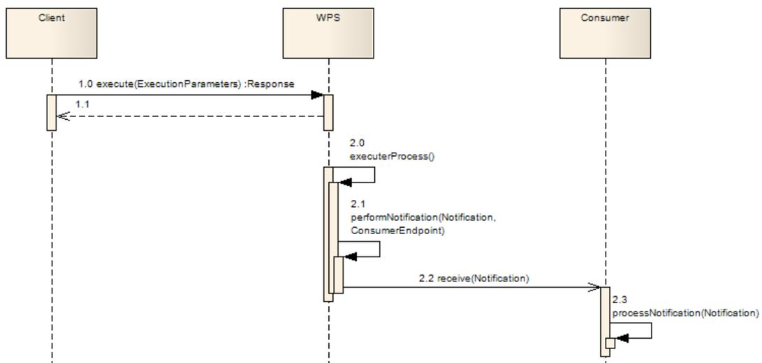
**Figure 35 - Exemplary sequence of interactions between a WPS, client and a consumer**
