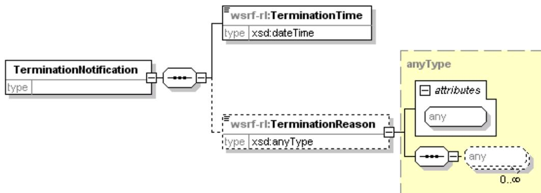
Figure 64 - TerminationNotification element in XMLSpy notation
