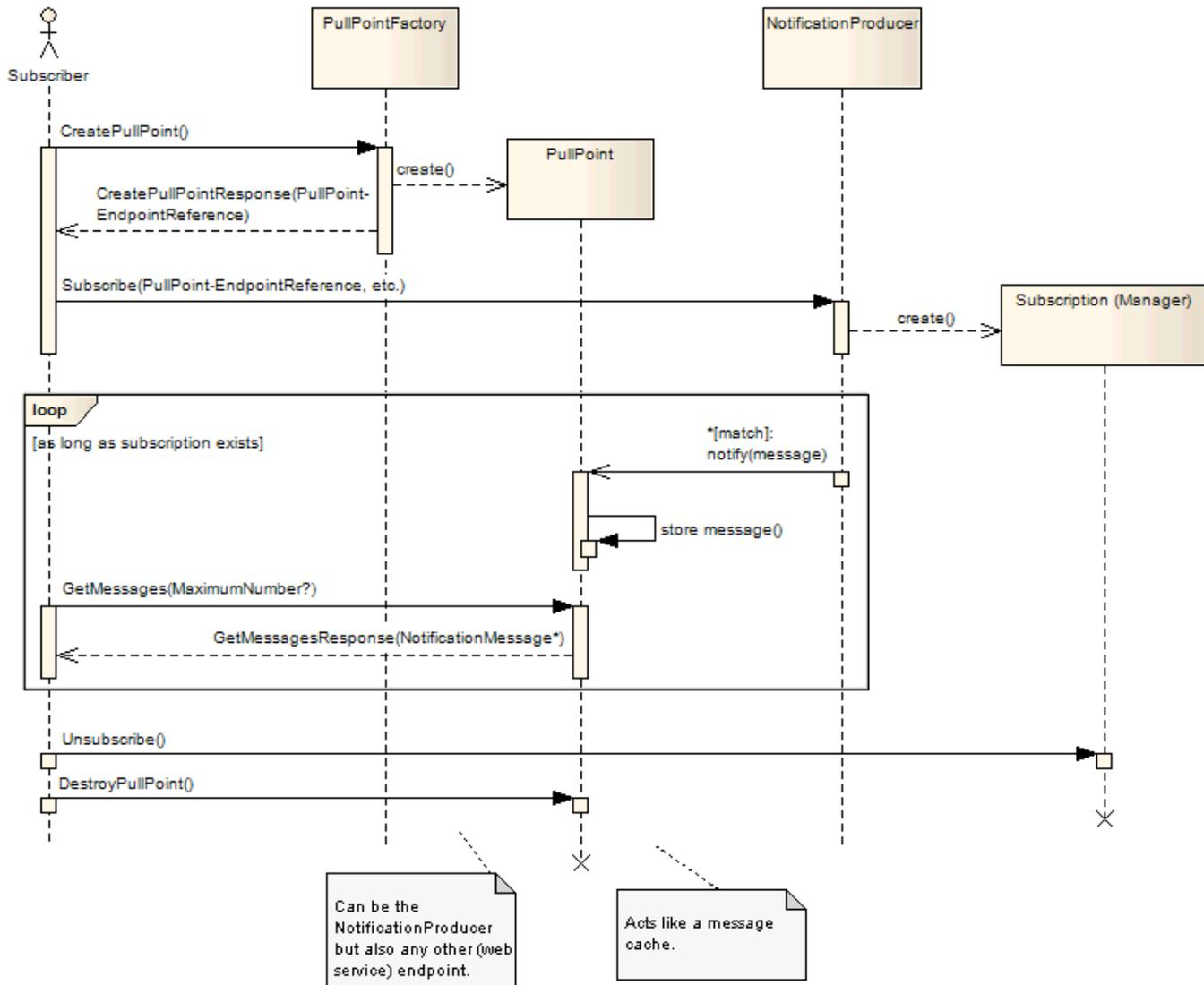
**Figure 75 – Pull style notification with WS-Notification using the PullPoint mechanism**
