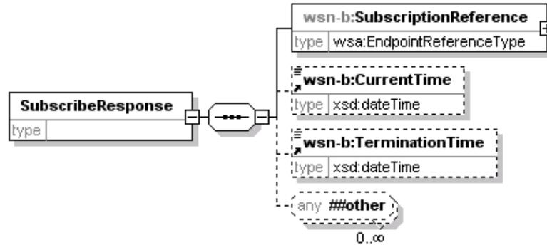
Figure 68 - SubscribeResponse element as defined by WS-BaseNotification in XMLSpy notation
