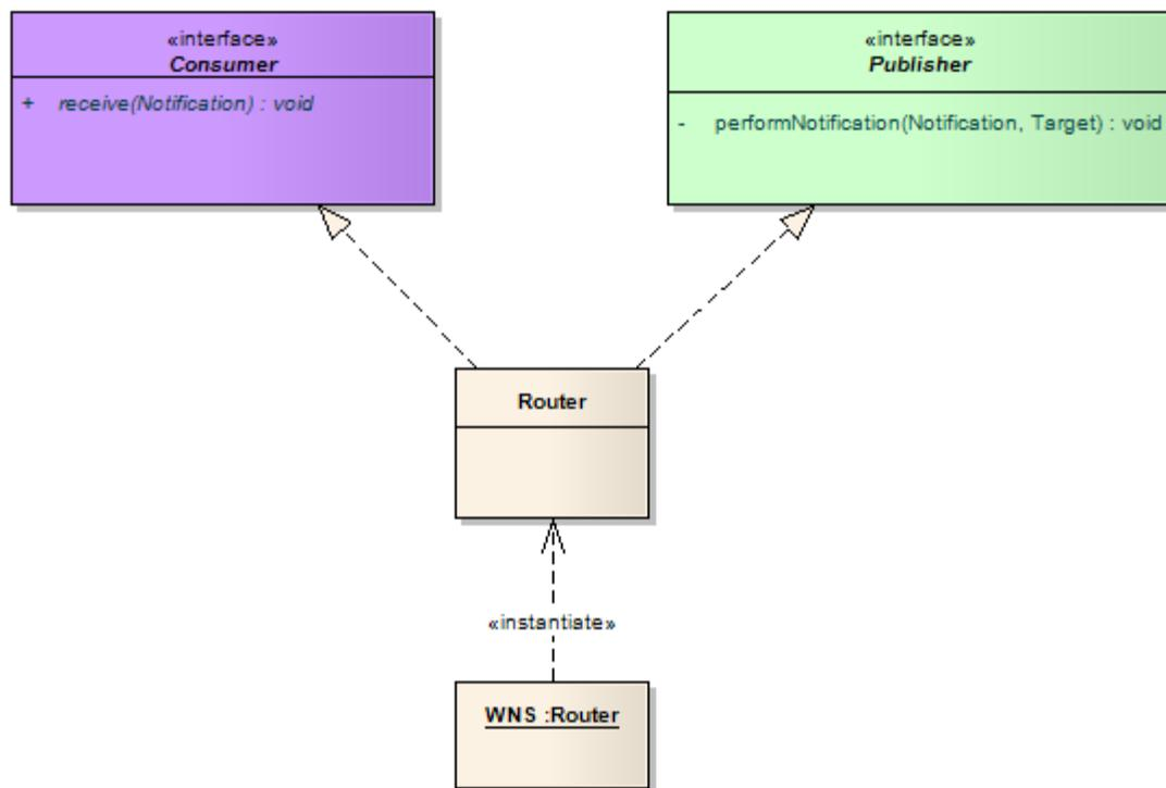
Figure 28 - Mapping the Router role to a WNS
