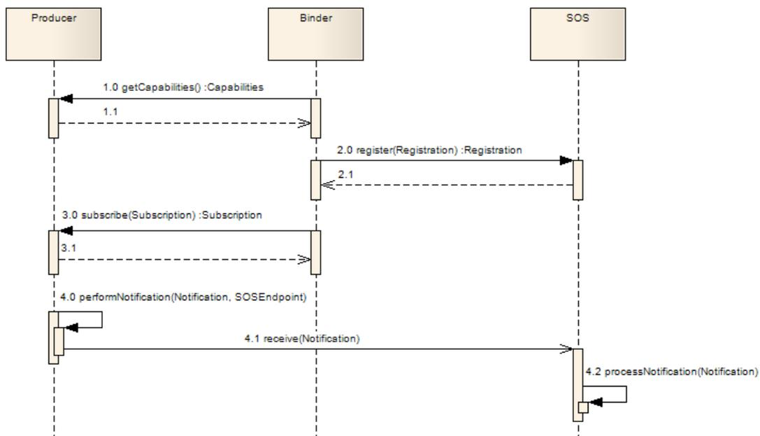
Figure 18 - Exemplary sequence of interactions between a SOS, binder and producer
