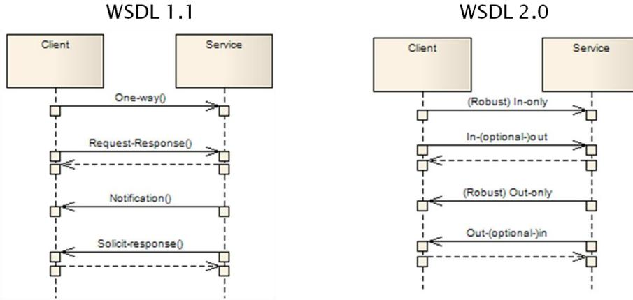
Figure 53 - Message Exchange Patterns described by WS-Addressing
