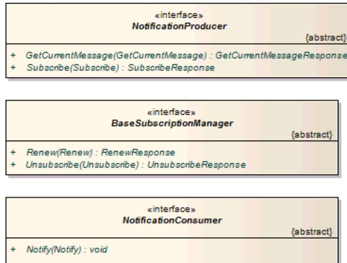
Figure 65 - Mandatory Interfaces defined by WS-BaseNotification
