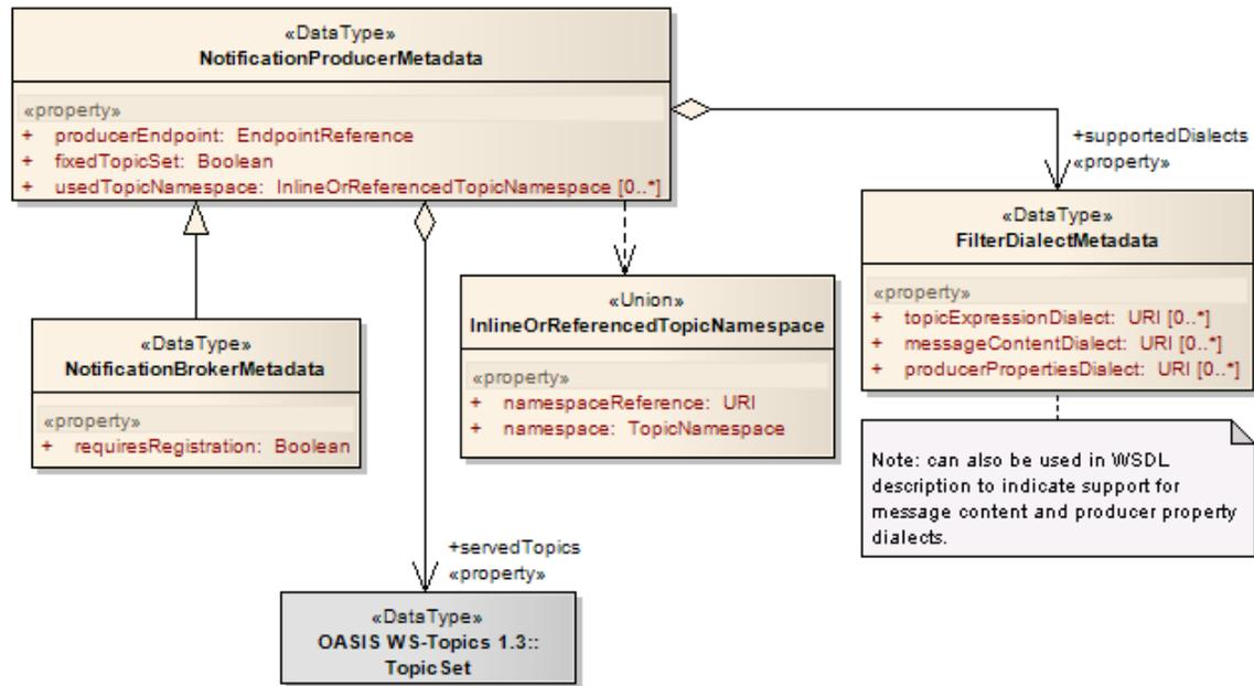
Figure 78 - Notification Metadata Data Types for inclusion in an OWS's Capabilities Document
