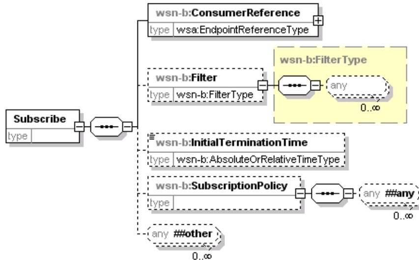
Figure 67 - Subscribe request element as defined by WS-BaseNotification in XMLSpy notation
