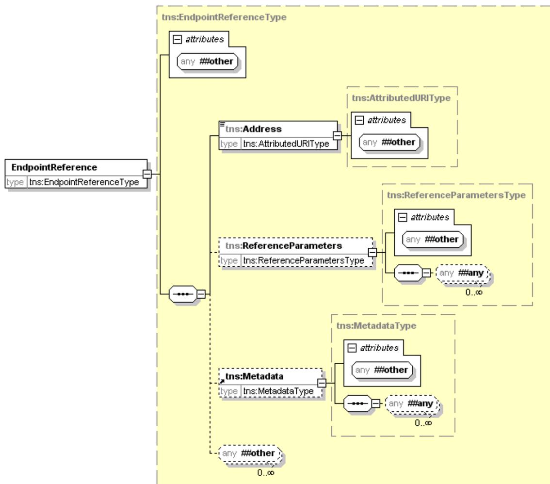
Figure 51 - WS-Addressing EndpointReference in XMLSpy notation
