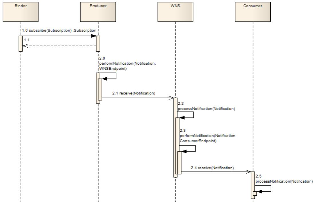
**Figure 29 - Exemplary sequence of interactions between a WNS, client, binder and producer**
