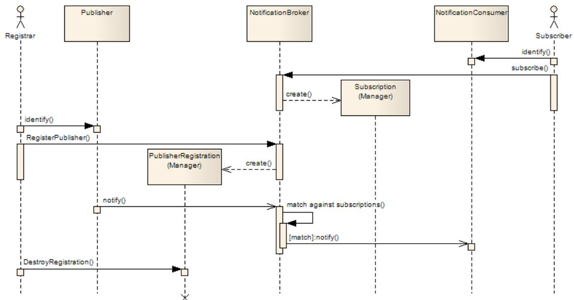
Figure 77 - Interactions in brokered Pub/Sub using WS-Notification
