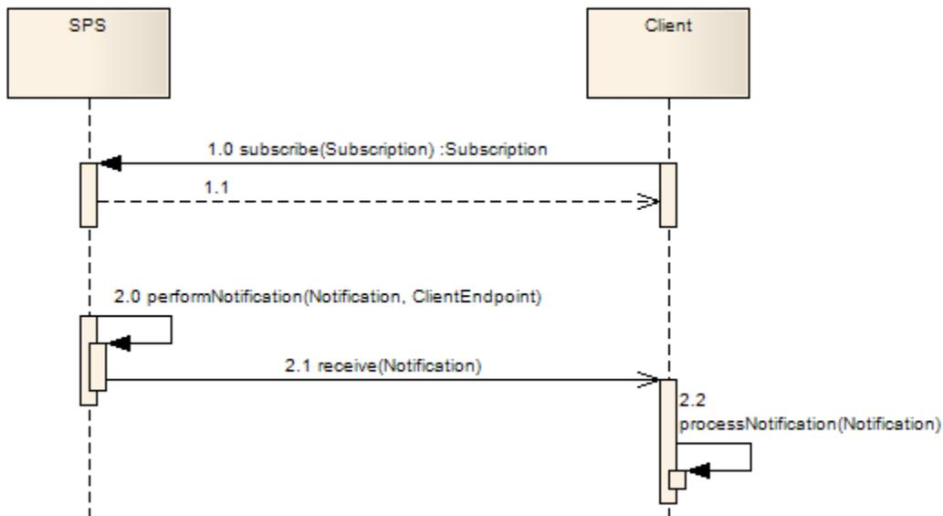
Figure 26 - Exemplary sequence of interactions between an SPS and a Client
