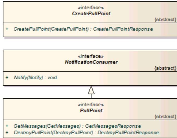
**Figure 74 - PullPoint interfaces as defined by WS-BaseNotification**
