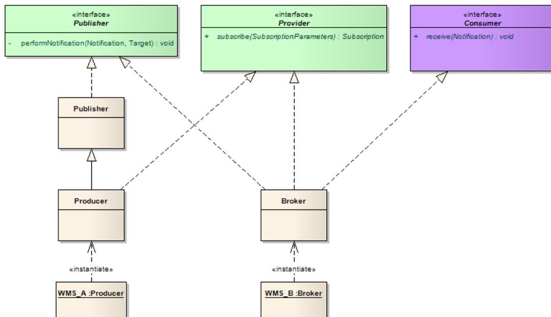
Figure 37 - Mapping the Producer and Broker role to WMSs
