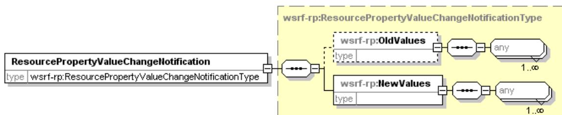
Figure 63 - ResourcePropertyValueChangeNotification element in XMLSpy notation
