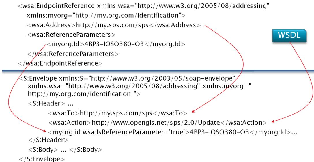
**Figure 52 - Handling of WS-Addressing MessageProperties**
