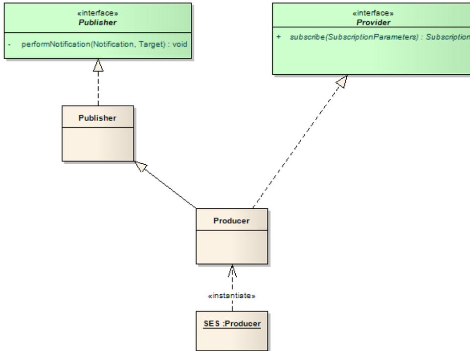
Figure 19 - Mapping the Producer role to a SES
