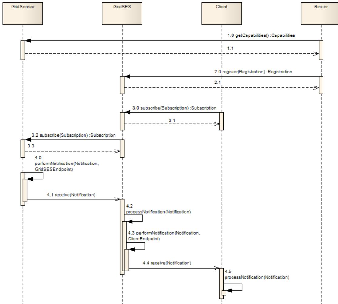
**Figure 23 - Exemplary sequence of interactions between a SES and sensor providing gridded data, a client and a binder**
