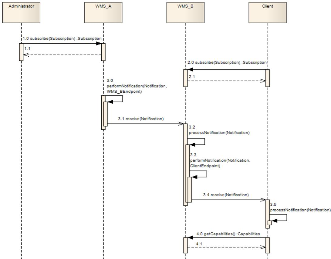
**Figure 38 - Exemplary sequence of interactions between two WMS, a client and an administrator**
