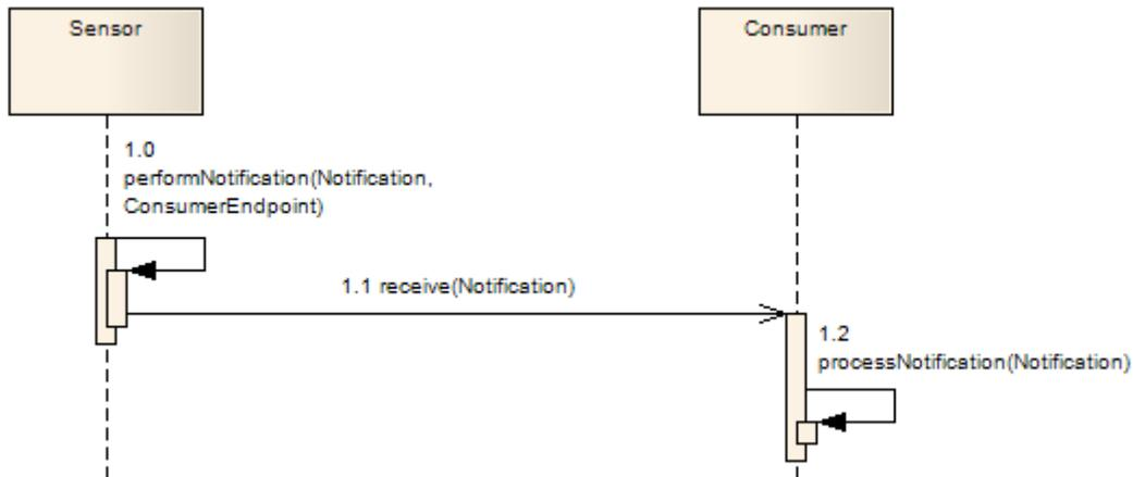
**Figure 15 - Exemplary sequence of interactions between a sensor and a consumer**
