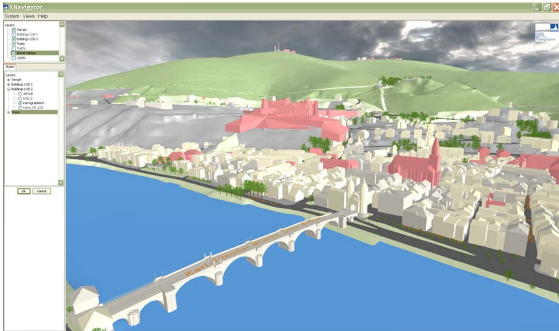
Fig. 7 Different building types are styled thematically using SLD 3D in a W3DS. (data sources: Bureau of Surveying, Stadtvermessungsamt Heidelberg, EML, own data)
