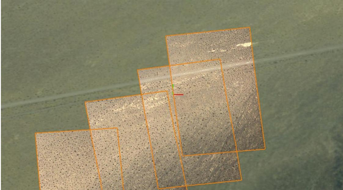
**Figure 11. On-demand geolocation of the GSI KSM-HD High-Definition video imagery taken from the Tigershark UAV during Empire Challenge 08; uses the SensorML encoding of the CSM Frame Sensor model along with the UAH Open Source SensorML process execution engine software.**
