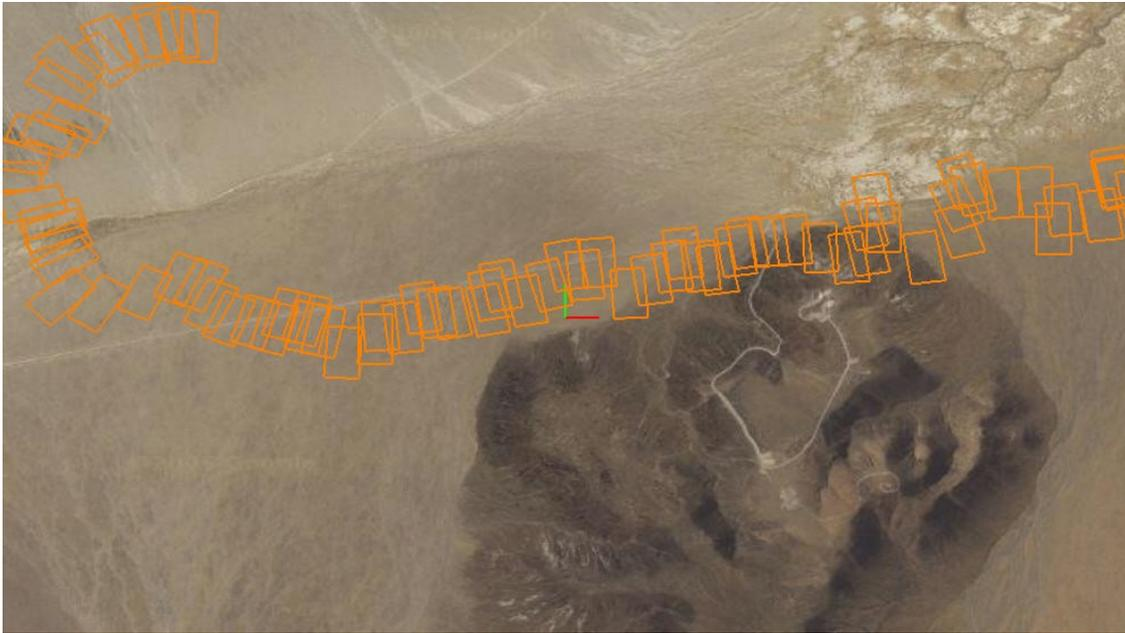
**Figure 12. Footprints calculated using a SensorML-encoded CSM Frame Sensor Model, based on retrieving the platform’s navigation data (i.e. location and attitude) from an SOS. Rather than treating such data as metadata for the imagery, treating sensor model parameters and other measurements as observations in their own right, enables increased capabilities for discovery and alerts.**
