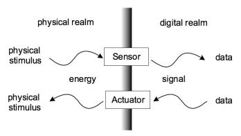
Figure 5-2: Sensor and actuator model (derived from (Ricker/Havens, 2005))
