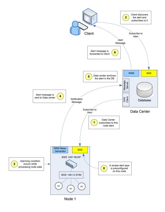
Note that if the data center **always** listens to **all** alerts coming from this node, step 1 is not necessary and the notification can be issued systematically by the node software. However, adding a real SAS interface to the node provides more flexibility since different network entities will be able to subscribe to different alerts. This could be of interest if the
