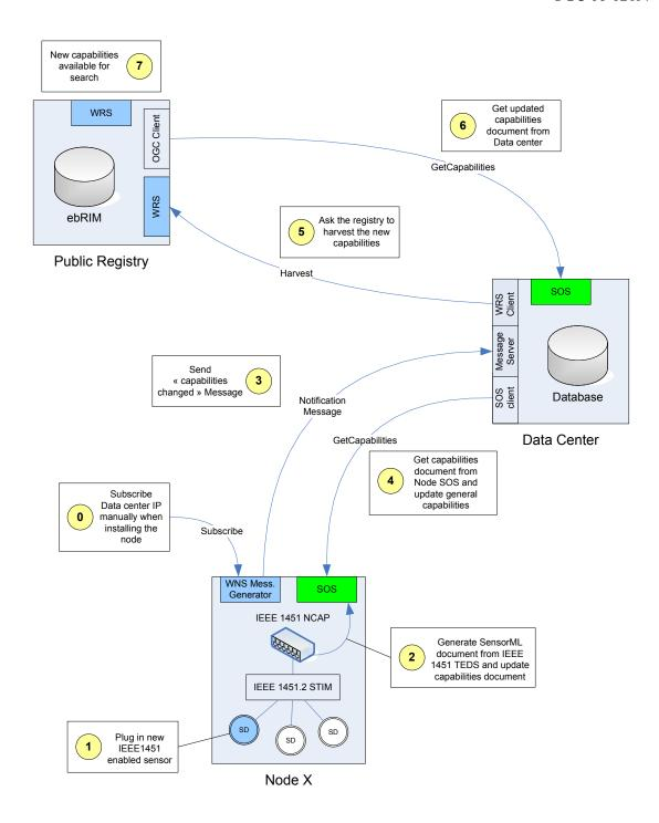
The next diagram illustrates how individual nodes can insert there observations in the main database using the data center SOS-T interface. This way of operation is very useful when nodes cannot keep a permanent network connection with the data center (e.g. GSM).
