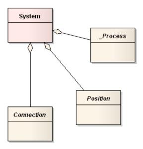
Figure 7-2. SensorML System aggregates processes, components, or data sources and describes their position and connnection
