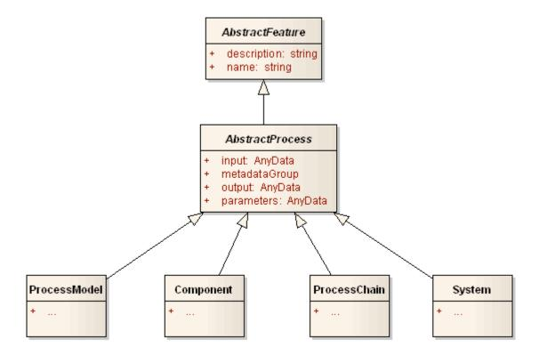
Figure 2. SensorML process types
