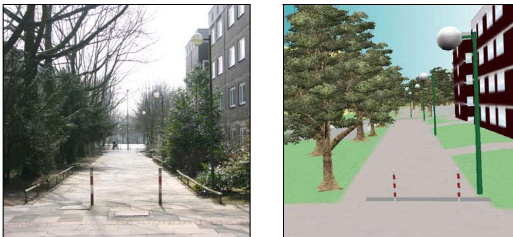
Fig. 43: Real situation showing lanterns and delimitation stakes (left). In the right image they are modelled as CityFurniture objects with ImplicitGeometries (source: 3D city model of Barkenberg).
