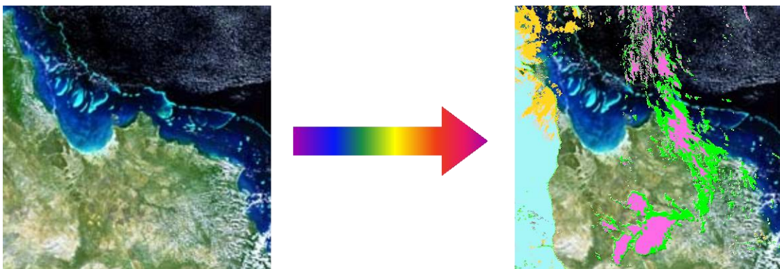
Figure 7-4: Application of four bitmasks to an EO dataset coverage false colour composite map. Note that four contrasting colours have been chosen to represent the bitmasks.
