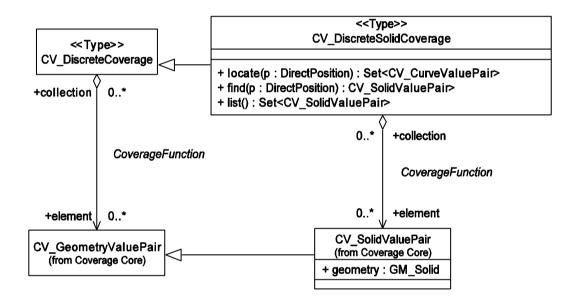
Figure 10 — CV\_DiscreteSolidCoverage
