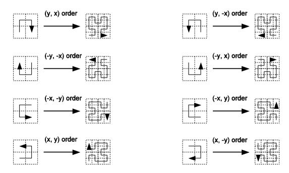
Figure D.7 — Replacement patterns for generating a Hilbert curve
