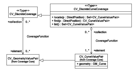
Figure 8 — CV DiscreteCurveCoverage
