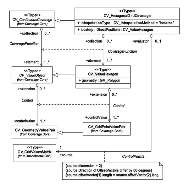
Figure 21 — CV\_HexagonalGridCoverage
