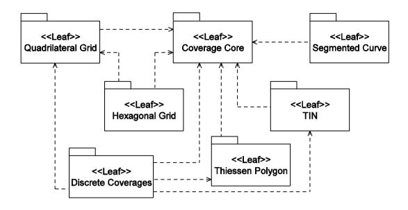
Figure 1 — Packages of the coverage schema
