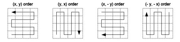
Figure D.2 — Examples of boustrophedonic scanning in a 2-dimensional grid
