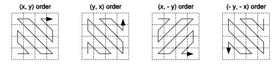
Figure D.3 — Examples of Cantor-diagonal scanning in a 2-dimensional grid
