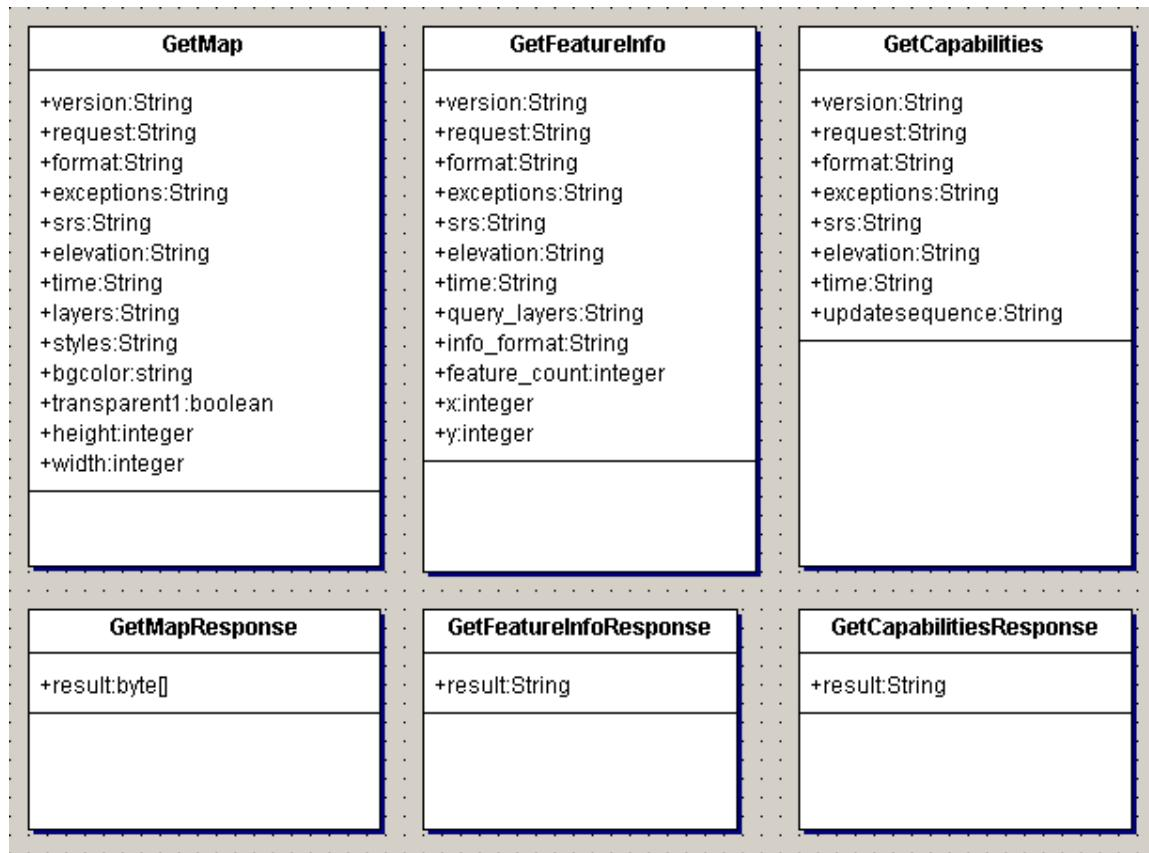
Figure 2: UML model for WMS HTTP Get Binding
