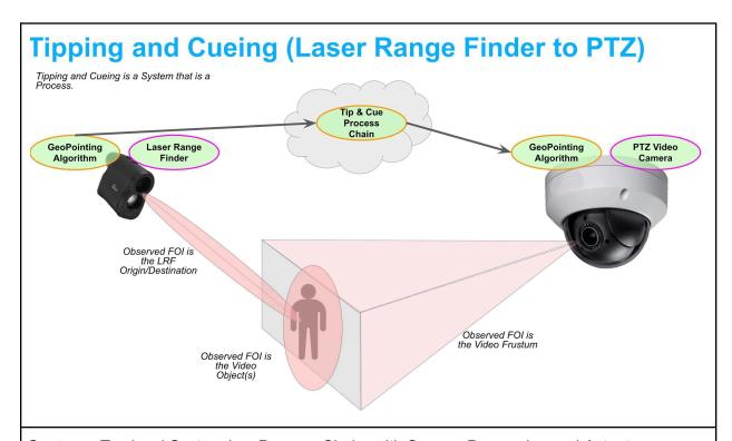
System: Top level System is a Process Chain, with Sensor, Processing and Actuator
