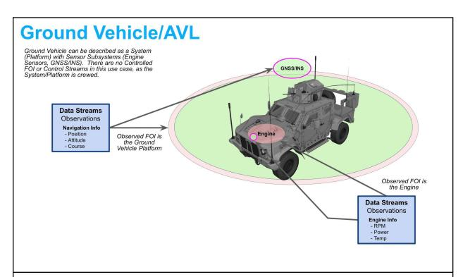
**System:** Ground Vehicle (the top level System is the Platform in this case)
