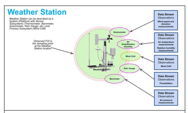
**System:** Weather Station (the top level System is the Platform in this case)
