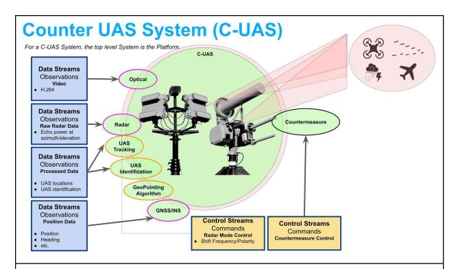
**System:** C-UAS System **Platform:** C-UAS System
