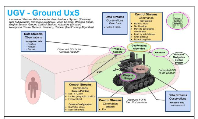
System: Ground UxS (Unmanned Ground System) (the top level System in this case includes
