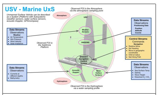
**System:** Marine UxS (Unmanned Surface Vehicle) **Platform:** USV (Unmanned Surface Vehicle)
