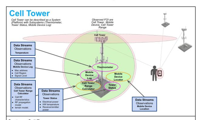
**System:** Cell Tower **Platform:** Cell Tower
