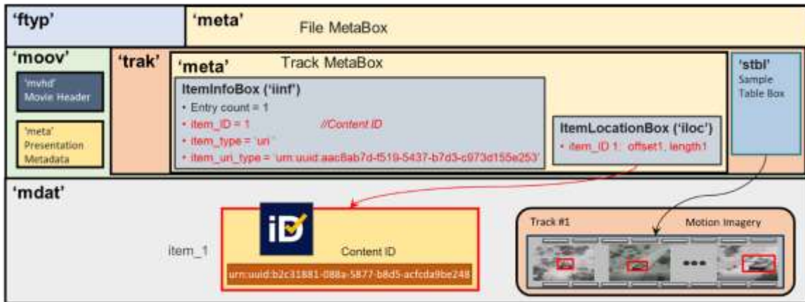
Figure 15: Attachment of a Content ID to a Motion Imagery track
