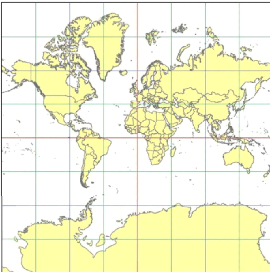
Figure 15. Tile Matrix Id 1 (red lines; 2x2 tiles) and 3 (blue lines; 8x8 tiles) of the WorldMercatorWGS84Quad TileMatrixSet (Source NGA)
