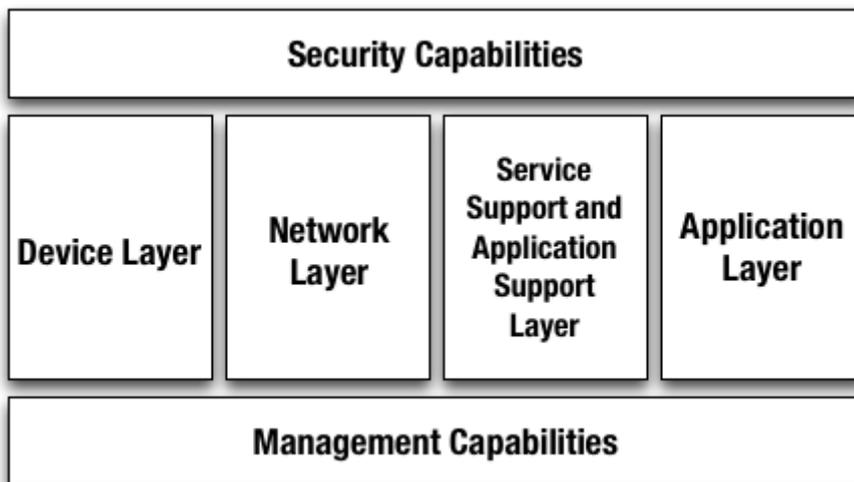
Figure 1. IoT Reference Model (adapted from [ITU-T Y.2060])
