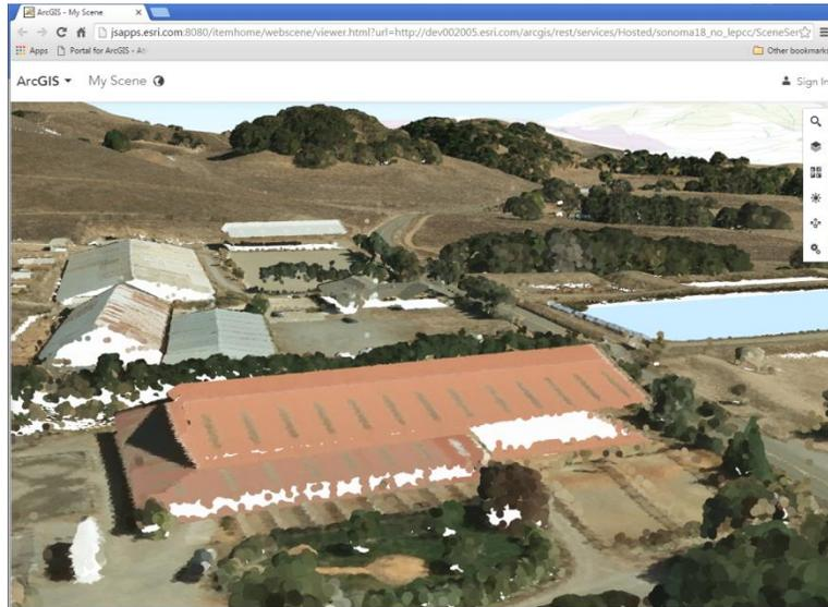
Figure 4: LiDAR-collected Point Cloud displayed in a web browser as a scene layer
