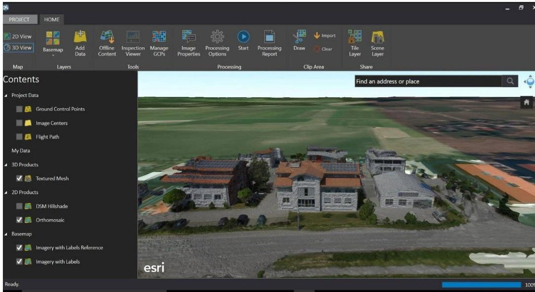
Figure 22. Esri Drone2Map can be used to create I3S integrated mesh content from drone-collected imagery
