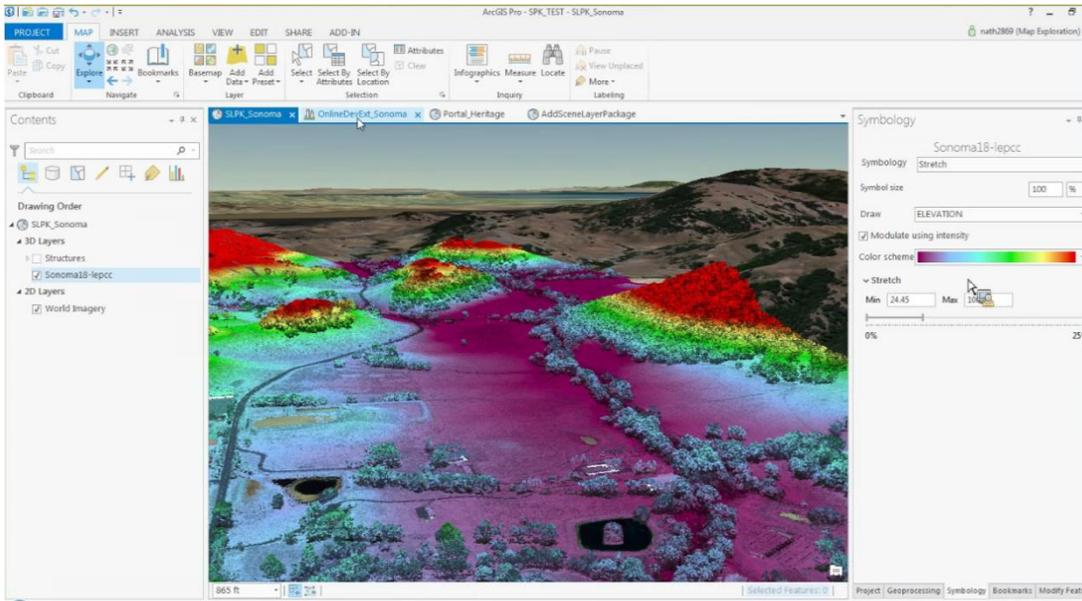
Figure 18. ArcGIS Pro 1.4 prerelease displaying a point clouds scene layer package
