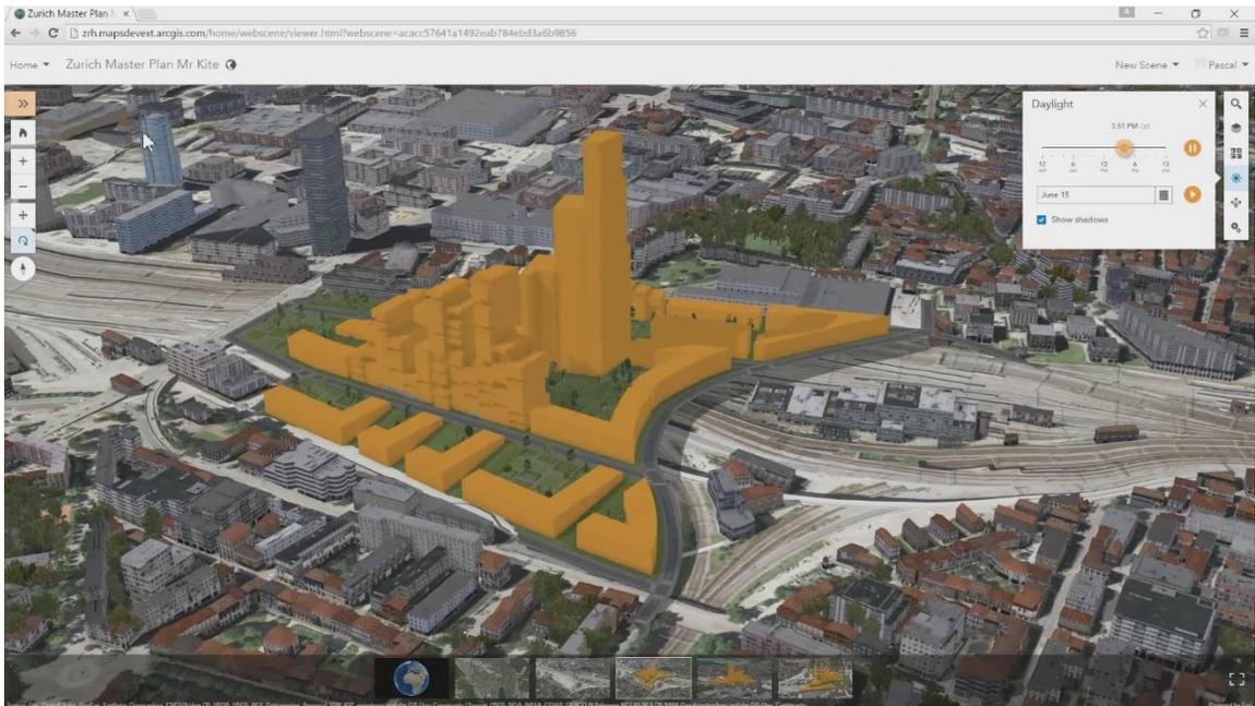
Figure 27. 3D model from CityEngine shown after being exported as a scene layer package and loaded in a web scene in ArcGIS Online
