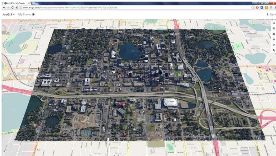
Figure 2. Integrated mesh scene layer from Bentley Systems' ContextCapture showing in a web scene.
