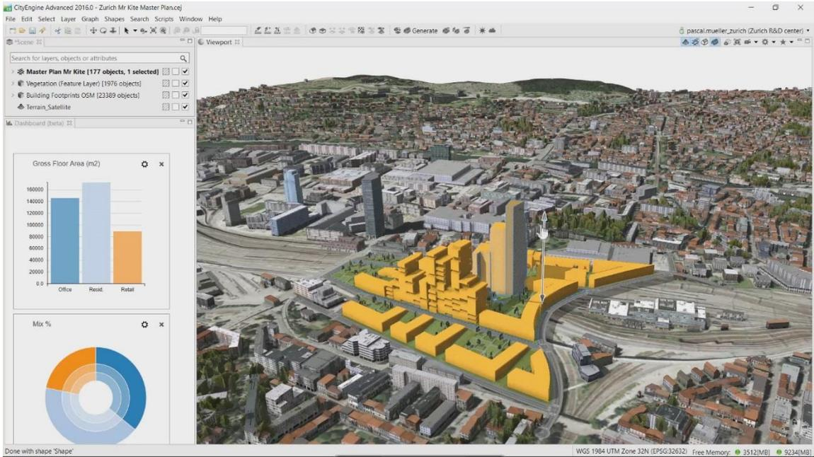
Figure 26. CityEngine shown being used to prepare data for export as a scene layer package file
