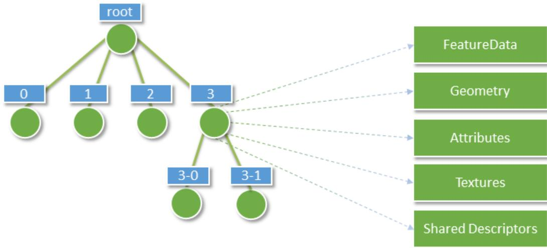
Figure 12: Per-node I3S resources: Feature-Data, Geometry, Attributes, Textures, Shared-Descriptors
