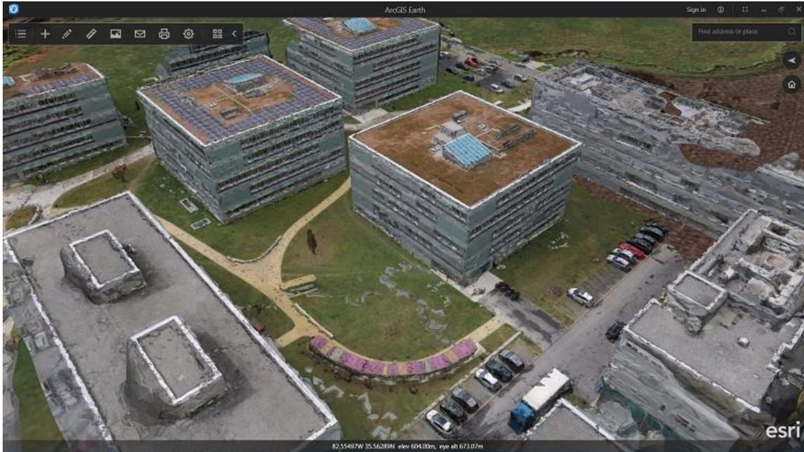
*Figure 21: ArcGIS Earth showing an integrated mesh scene layer that was created in Drone2Map and shared using ArcGIS Online.*
