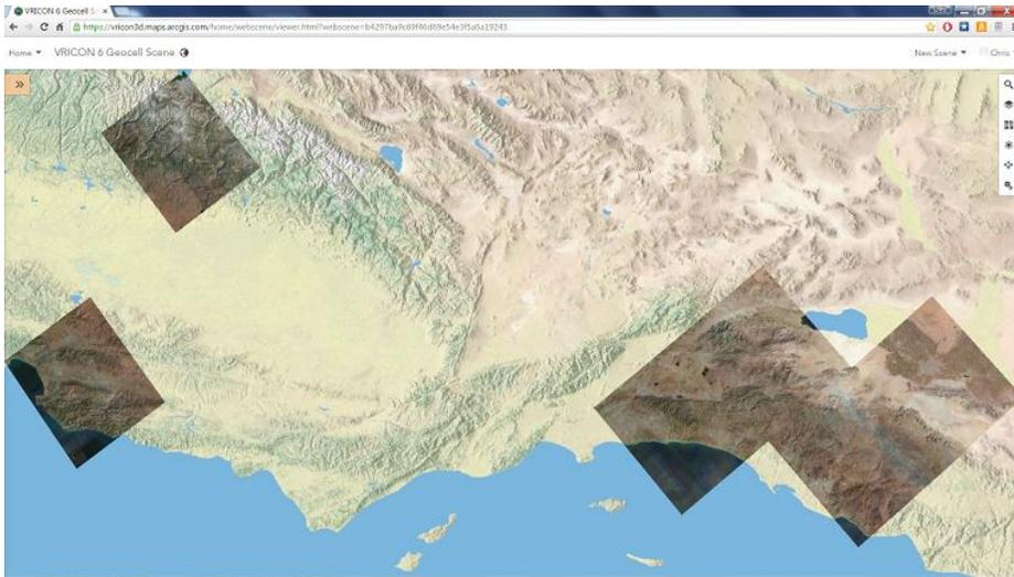
*Figure 9. Web scene showing six Vricon geocells covering approximately 60,000 sq km and totaling over 400GB of disk space in packaged format*
