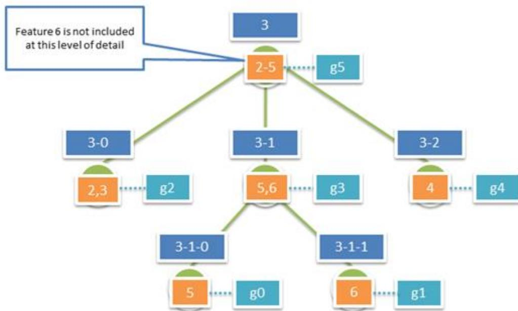
Figure 13: Example Nodes in a Mesh Pyramid. Orange boxes represent features stored explicitly within the node, the numbers represent feature identifiers. Turquoise boxes represent the geometry instances associated with each node – each geometry instance is an aggregate geometry (a geometry collection) that covers all the features in the node.
