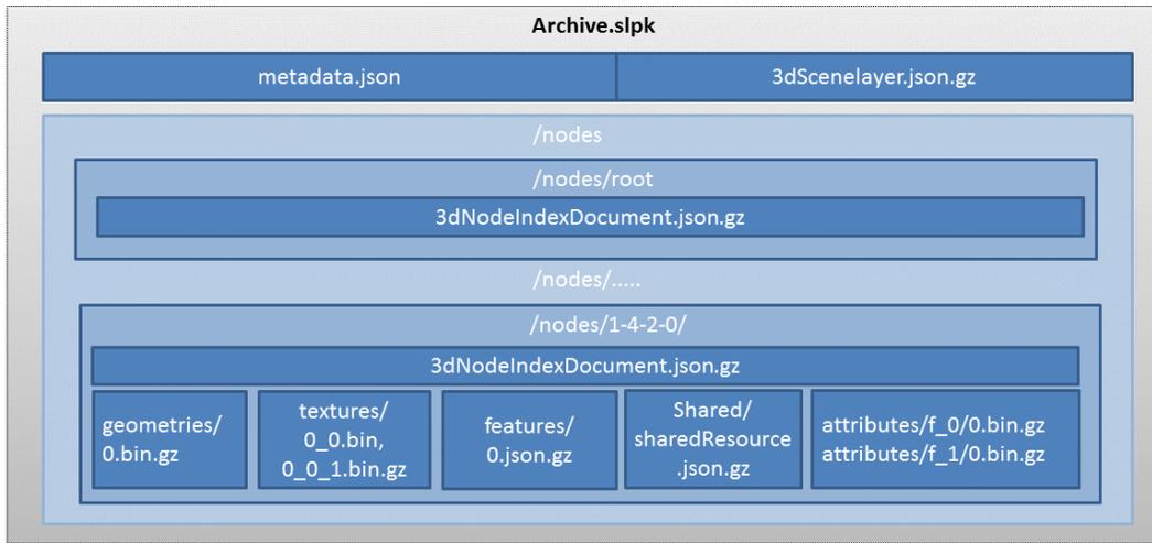
Figure 15: An example of a Scene Layer Package with its structure.
