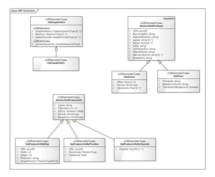
Figure 1: 3DPS UML class diagram
