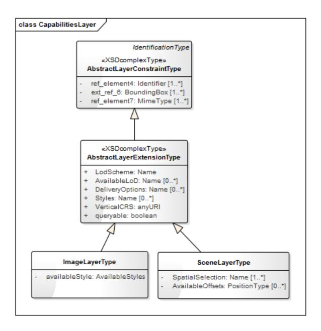
Figure 5: 3DPS core:Contents and core:Layer and UML class diagram
