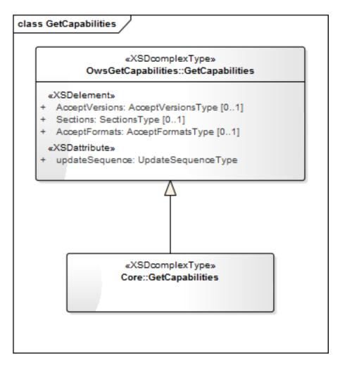
Figure 3: 3DPS core:GetCapabilities request UML class diagram
