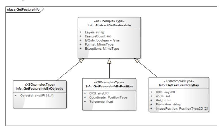
Figure 18: 3DPS info: AbstractGetFeatureInfo operation request UML class diagram
