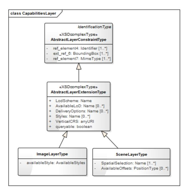
Figure 14: 3DPS view: Layer extensions UML class diagram
