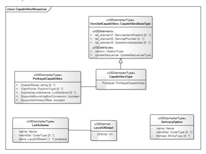
Figure 4: 3DPS Capabilities UML class diagram
