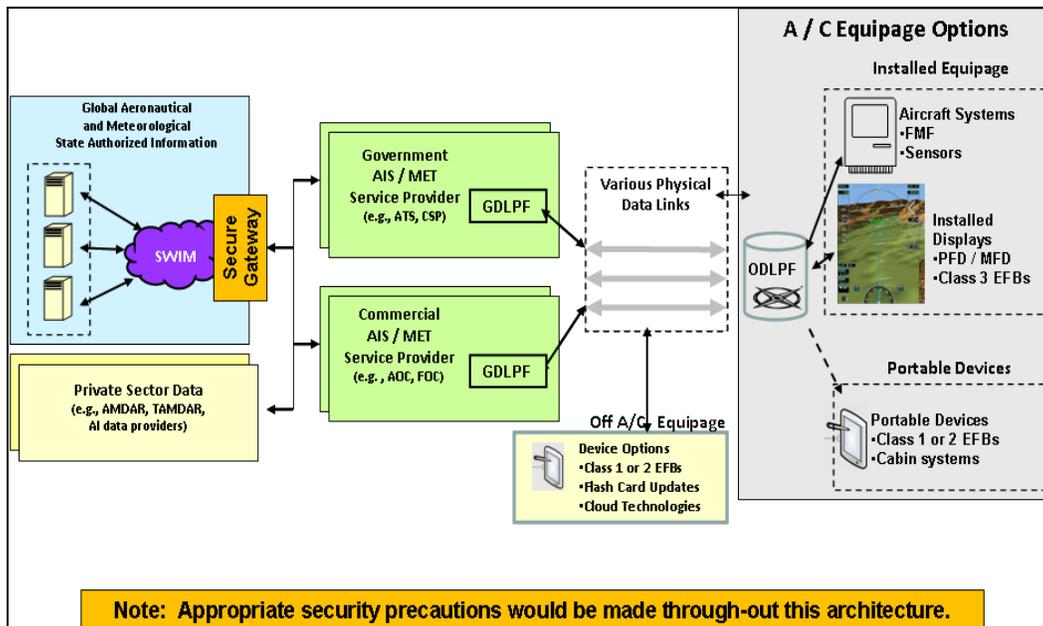
**Figure 7 - AIS and MET services physical architecture (notional) (Source: RTCA DO-340)**
