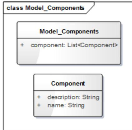
Figure 12: UML diagram of the model components definition
