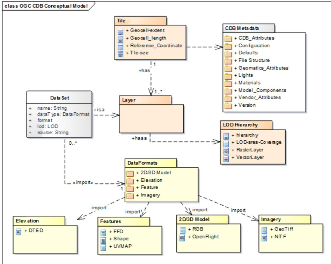
Figure 1: Package diagram of OGC CDB data store conceptual model
