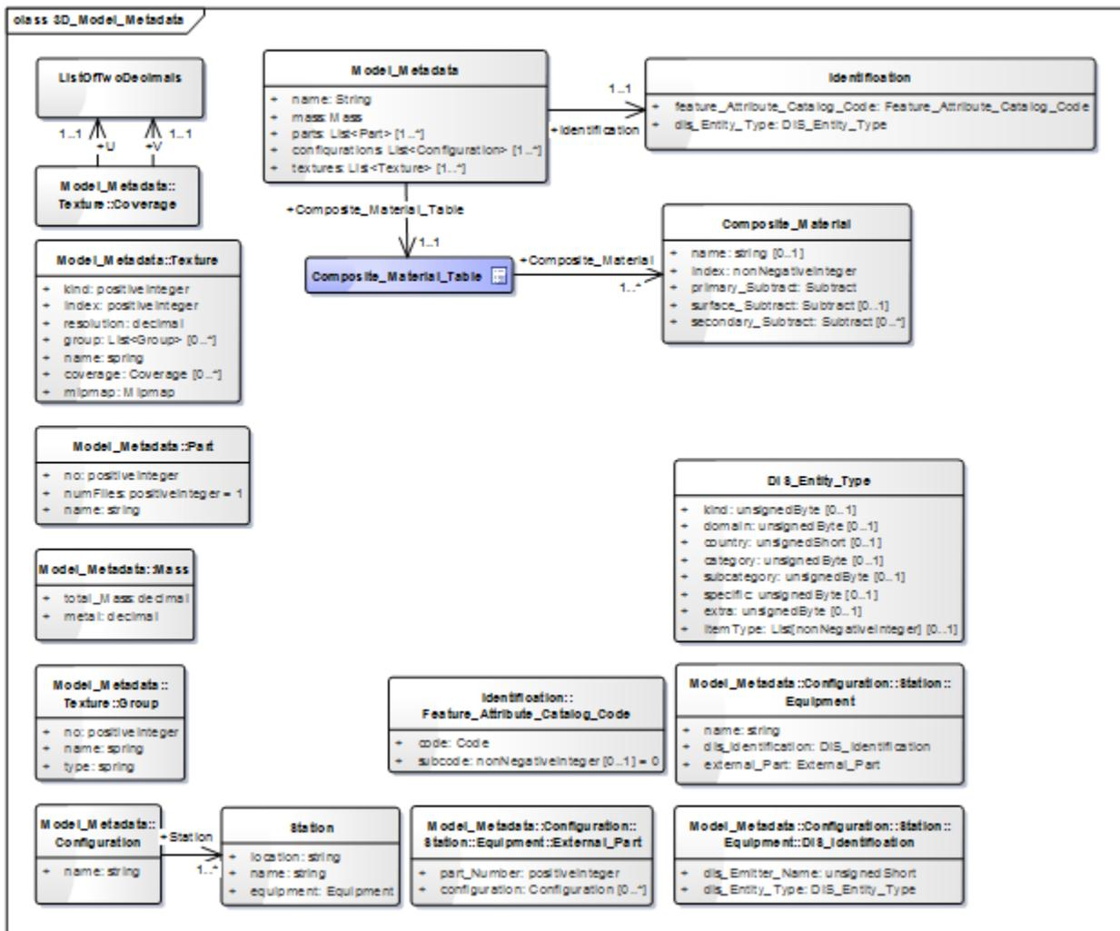
Figure 19: UML diagram of 3D model metadata
