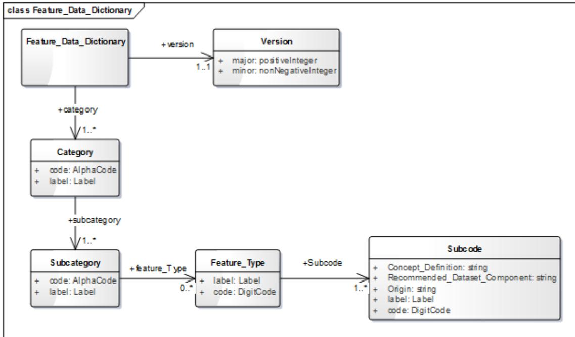
Figure 21: UML diagram of feature data dictionary
