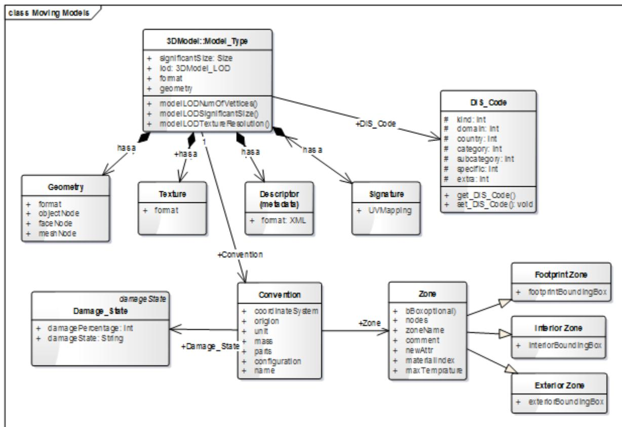
Figure 7: UML diagram of the 3D moving model
