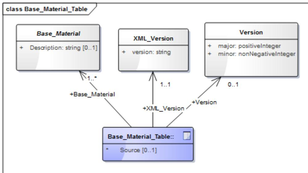
Figure 13: UML diagram of the base materials table
