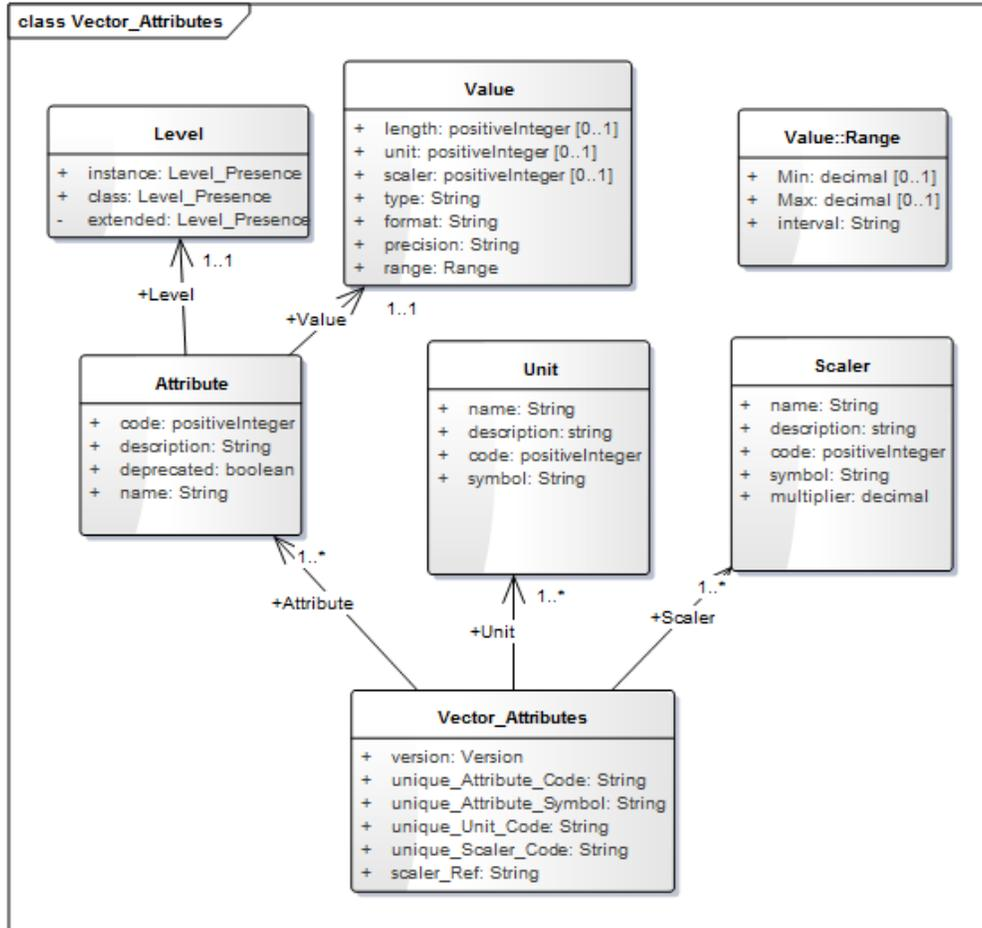
Figure 18: UML diagram of the CDB vector attributes
