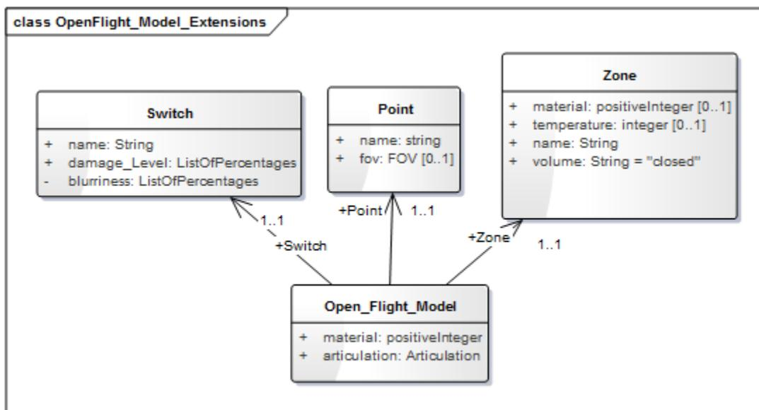
Figure 20: UML diagram of OpenFlight model extensions
