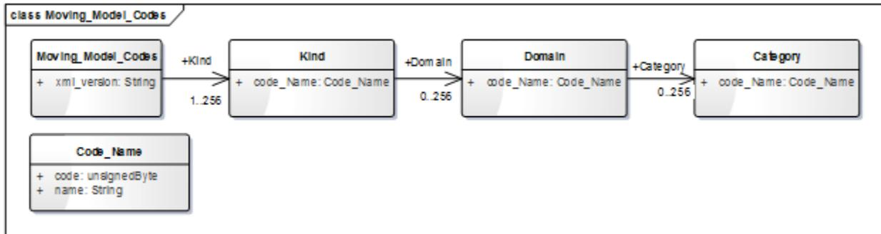
Figure 8: UML diagram of moving model codes
