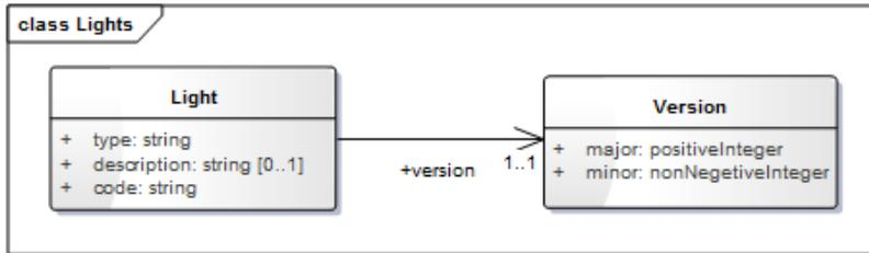
Figure 10: UML diagram of light names hierarchy
