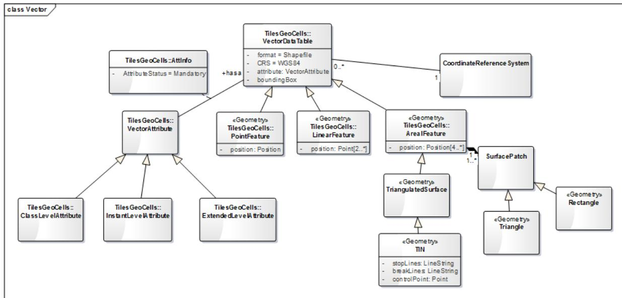
Figure 9: UML diagram of vector data model
