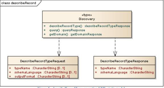
Figure 5 - describeRecordType operation UML static model
