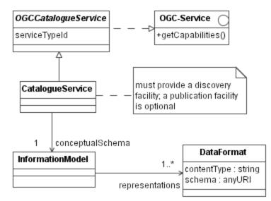
Figure 10 - Application profiles specify concrete catalogue services
