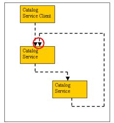
Figure 14 - Query network topology resulting in closed loops
