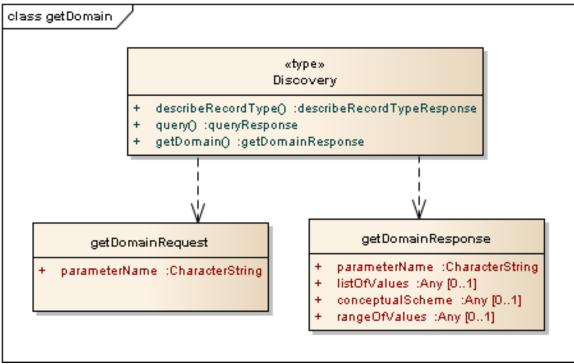
Figure 6 - getDomain operation UML static model
