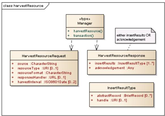
Figure 8 - harvestResource operation UML static model
