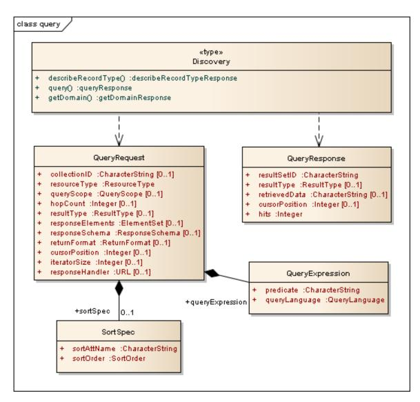
Figure 4 - "query" operation UML static model
