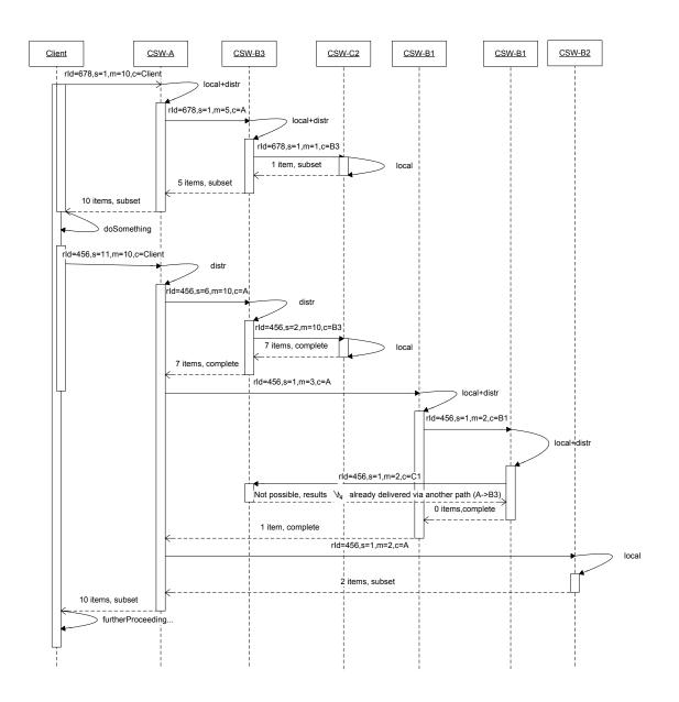
Figure 18 - Distributed Search Example (sequence diagram)
