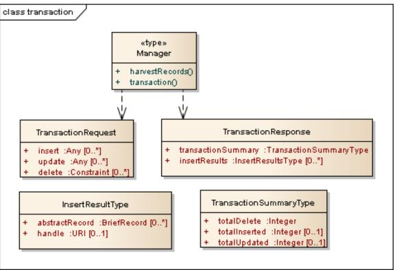
Figure 7 - "transaction" operation UML static model
