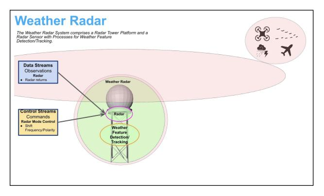
System: Weather Radar System Platform: Radar Tower Sensors: Radar Actuators: None Processes: Weather Feature Detection/Tracking Features of Interest: Radar, Radar Lobes, Targets (aircrafts / drones / birds / weather) Data Streams/Observations: Raw radar data (echo power at azimuth/elevation), Processed data = reflectivity (etc.) coverage, additional processing to get features Control Streams/Commands: Radar Mode (shift frequency/polarity, elevation/azimuth speed/increments)
