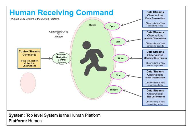
Sensors: Eyes, Ears, Nose, Skin, Tongue Actuators: Human legs, being told to go somewhere and sense/do something. Processes: None Features of Interest: Object Data Streams/Observations: None Control Streams/Commands: Location to move to received by the human
