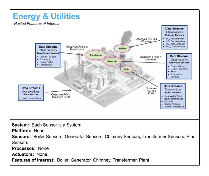
**Data Streams/Observations:** Input Water Temp, Boiler Temperature, O<sub>2</sub> Level, Steam Pressure, Steam Temperature (Boiler); Output Voltage, Output Frequency, RPM, Temperature, Vibration (Generator); SO<sub>2</sub>, NOx, PM<sub>10</sub>,PM<sub>2.5</sub> Concentration (Chimney); Terminal Voltage, Frequency, Power Factor, Temperature (Transformer); Total Power Output (Plant) **Control Streams/Commands:** None
