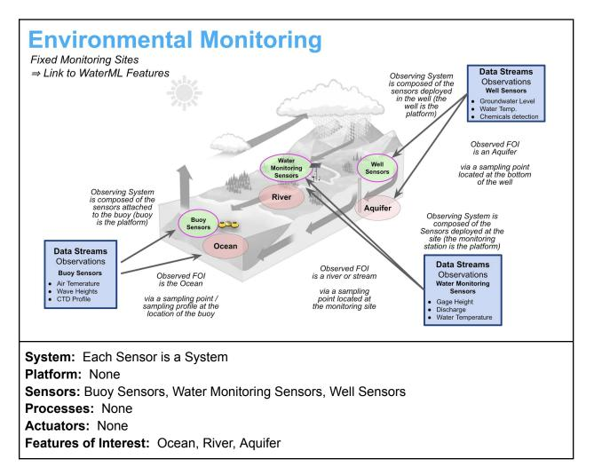
**Data Streams/Observations:** Air Temperature, Wave Heights, CTD Profile (Buoy Sensor), Gauge Height, Discharge, Water Temperature (Water Monitoring Sensors), Groundwater Level, Water Temperature, Chemicals detection (Well Sensors) **Control Streams/Commands:** None
