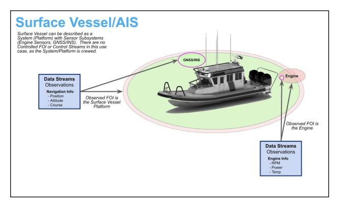
System: Surface Vessel (the top level System is the Platform in this case) Platform: Surface Vessel (the Platform is the top level System) Sensors: GNSS/INS, Engine Sensors (Subsystems mounted on the Platform) Actuators: None Processes: None Features of Interest: Surface Vessel, Engine Data Streams/Observations: Positioning Data, Engine Performance Control Streams/Commands: None
