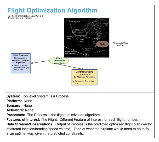
**Control Streams/Commands:** Set algorithm parameters for given flight ID (e.g. optimize for fuel and/or time); Trigger optimization on-demand (if not automatically triggered); In general, this would run on its own. But, it could also be triggered by a pilot/navigator at any time using an Execute Command, with some parameters beyond Flight ID.
