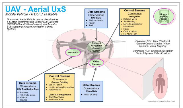
**System:** Unmanned Aerial System (UAS) (the top level System in this case includes the Platform and the Ground Control Station (GCS))
