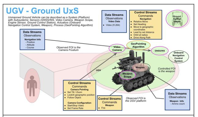
**System:** Ground UxS (Unmanned Ground System) (the top level System in this case includes the Platform and the Ground Control Station (GCS))
