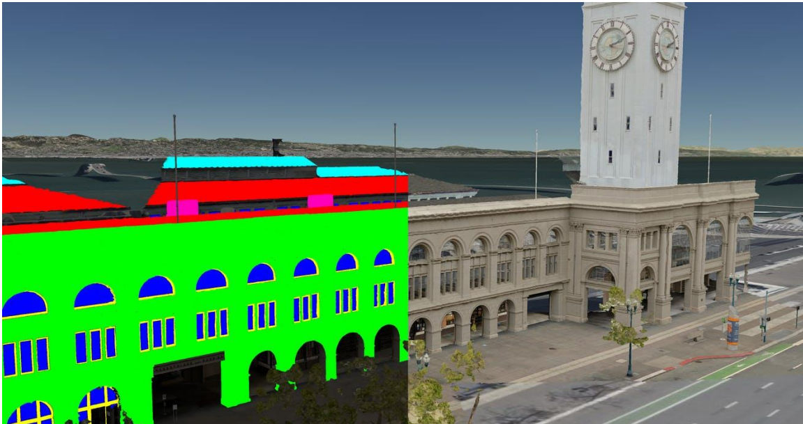
Street level photogrammetry of San Francisco Ferry Building from Aerometrex. Left: per-texel colors showing the feature classification, e.g., roof, sky roof, windows, window frames, and AC units . Right: classification is used to determine rendering material properties, e.g., make the windows translucent.
