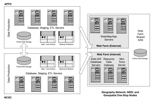
Figure 4.1: Computational architecture of the GDW.
